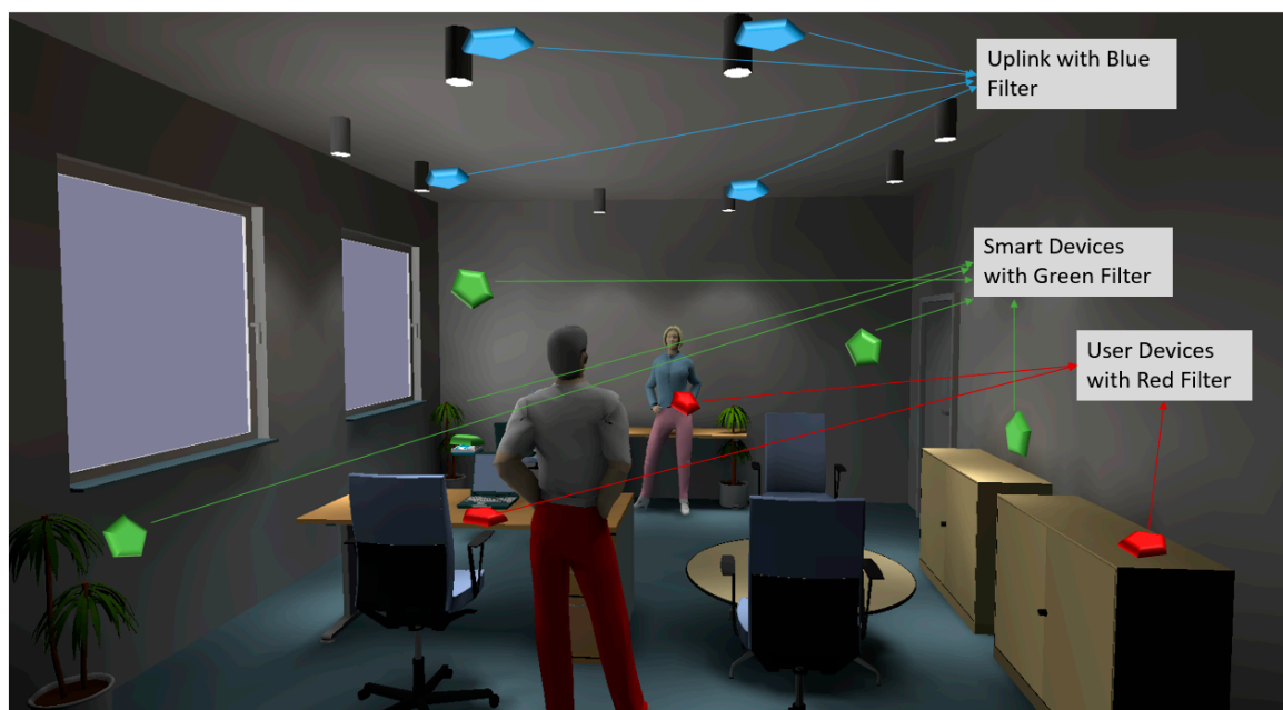
Figure 1. Proposed multi-user full-duplex visible light communication (VLC) system.
