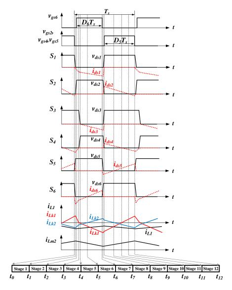
Figure 6. Key waveforms of the proposed converter in step-down mode.
