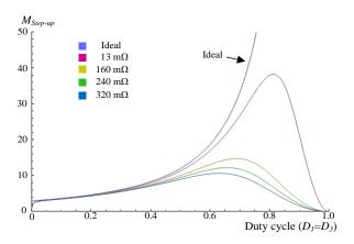
Figure 12. The step-up voltage gain under different choke resistances.
