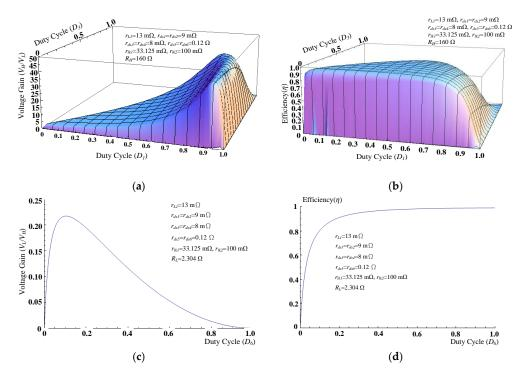
**Figure 11.** The relationships of voltage gain versus duty ratio and efficiency versus duty ratio while considering non-ideal effect: (a)  $M'_{step-up}$ ; (b)  $\eta_{step-up}$ ; (c)  $M'_{step-down}$ ; and (d)  $\eta_{step-down}$ .
