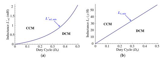
**Figure 9.** The relationship between the inductance and duty ratio  $D_6$ : (a)  $L'_{m2}$ ; and (b)  $L_1$ .
