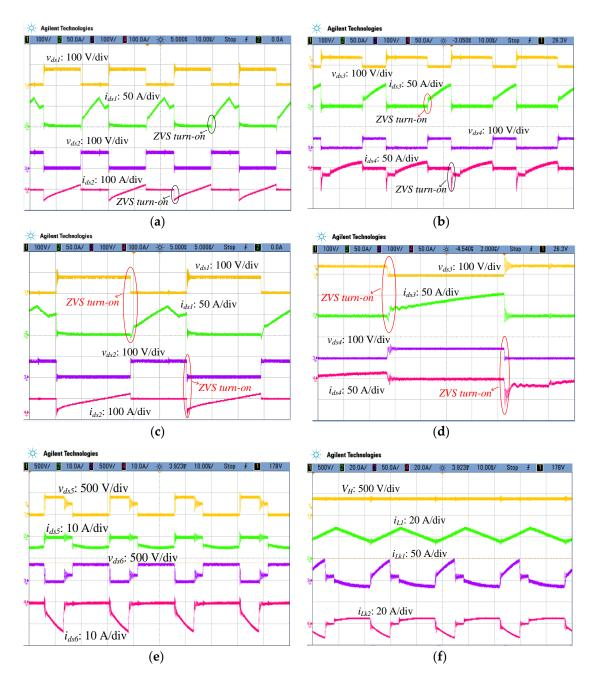
**Figure 13.** Experimental results in step-up mode operation at  $P_0 = 1$  kW: (a) measurements from  $S_1$  and  $S_2$ ; (b) measurements from  $S_3$  and  $S_4$ ; (c) zoomed-in waveforms measured from  $S_1$  and  $S_2$ ; (d) zoomed-in waveforms of  $S_3$  and  $S_4$ ; (e) measurements from  $S_5$  and  $S_6$ ; and (f) waveforms of  $V_H$ ,  $i_{L1}$ ,  $i_{Lk1}$ , and  $i_{Lk2}$ .
