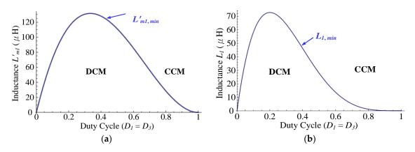
**Figure 7.** Magnetic component design for (a)  $L'_{m1}$  and (b)  $L_1$  under the duty ratio  $D_1 = D_3$ .
