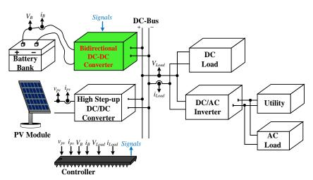
Figure 1. Configuration of distributed generation system.
