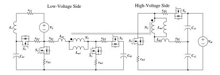
Figure 10. The non-ideal equivalent circuit of the converter.
