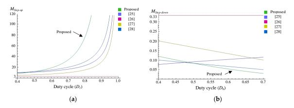
Figure 17. The comparison plots of conversion ratio: (a) step-up mode; and (b) step-down mode.
