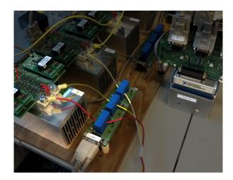
**Figure 7.** Photo of the single general purpose H-bridge used for driving the currents for system identification measurements, highlighted to the left. The current measurement board is seen in the middle, and the CompactRIO programmable automation controller used for sampling and storing of data is seen to the right.
