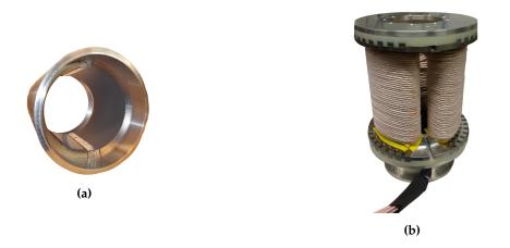
**Figure 3.** Photographs of rotor and stator of SRM prototype. (a) The assembled outer-rotor prototype, not including the central shaft. One half ferromagnetic and one half austenitic stainless steel; and (b) the three-phase stator with windings. The aluminum lid is on top, with a plastic plate separating it from the standing laminated c-shaped bits. The windings are wound around each of the three groups of c-shaped bits. The stator is hollow to allow for a shaft in the prototype.
