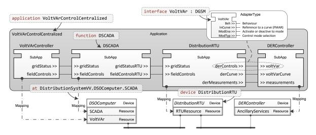
Figure 11. VoltVArControlCentralized as IEC 61499 Application<sup>499</sup>.
