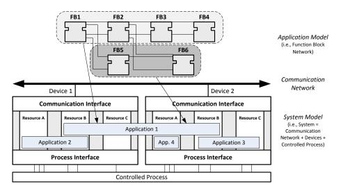
Figure 2. IEC 61499 reference models for distributed automation, based on [18,20].
