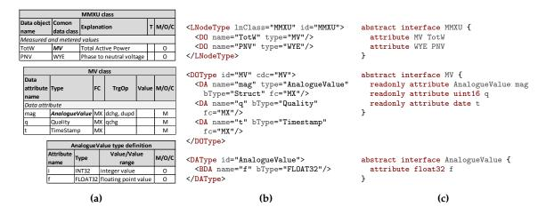
**Figure 9.** Mapping between an  $LN^{850}$  and an <interface>: (a) Excerpt of the  $LN^{850}$  MMXU in IEC 61850; (b) MMXU as SCL description; (c) MMXU as <interface> description.
