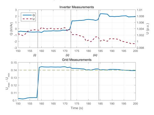
**Figure 15.** Measurements from the laboratory validation with three main events: (*i*) detection of voltage band violation, (*ii*) first curve correction, and (*iii*) second curve correction.
