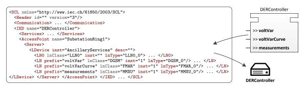
**Figure 14.** Generated System Configuration Language (SCL) file for configuration of the IEC 61850 server in *DERController*.
