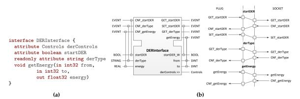
Figure 7. Illustrating example of a mapping between an <interface> and an Adapter<sup>499</sup>:
