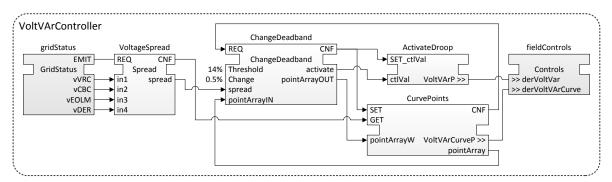
Figure 12. Implementation of the *VoltVArController* SubApp<sup>499</sup> from Figure 11.
