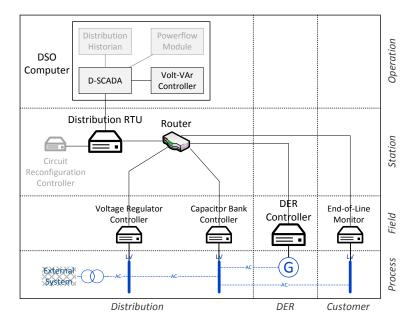
Figure 10. Overview of the example use case Integrated Volt VAr Control Centralized [46].
