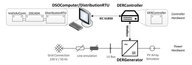
Figure 13. Laboratory setup for the use case validation.
