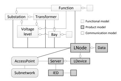
Figure 3. Main modeling objects as defined in IEC 61850-6, based on [21].
