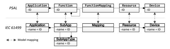
Figure 6. Mapping between IEC 61499 and PSAL for the component model.
