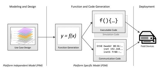
Figure 4. Conceptual view of the proposed rapid engineering methodology.
