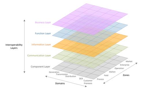
Figure 1. Overview of the Smart Grid Architecture Model (SGAM), based on [14].
