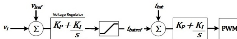
Figure 8. Battery SoC control diagram.
