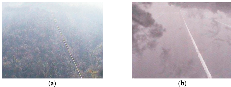
Figure 2. The color images are captured from a fixed remote camera, whose image size is 640*480. (a) A color image of an un-iced power transmission line; (b) A color image of an iced power transmission line.
