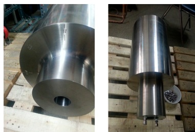
Figure 9. CEDM nozzle specimen with a J-groove weld.
