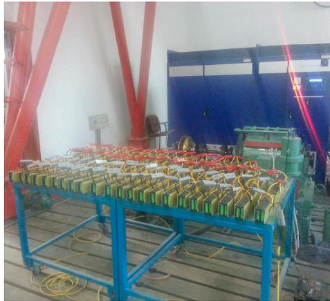
Figure 10. Battery pack and electronic load.
