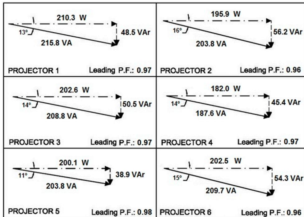
**Figure 3.** Power consumption triangles (Horizontal: active power (W). Vertical: reactive/inductive power (VAR). Diagonal: total/apparent power (VA)) measured with the 6 LED projectors used in this field-test.
