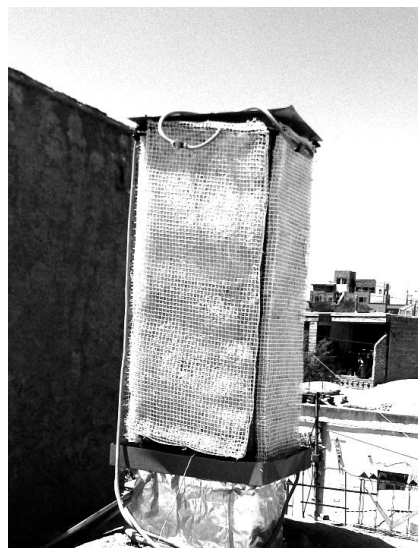
Figure 7. View of the manufactured wind tower head with wetted surfaces.
