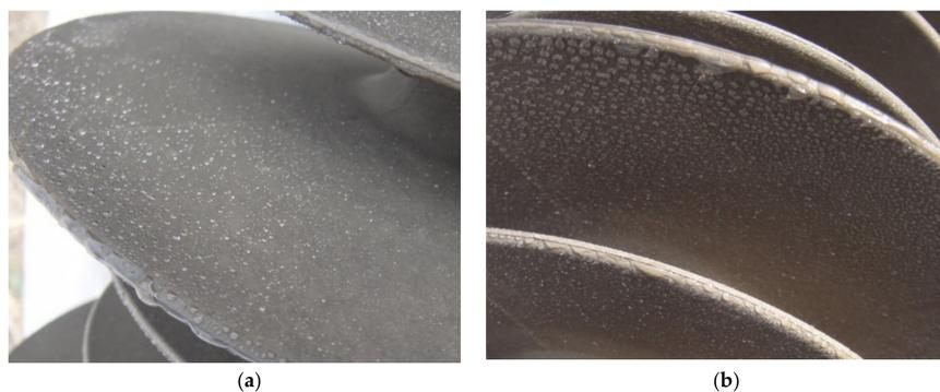
**Figure 13.** The hydrophobicity of the composite insulators. (a) The upper surface; (b) the lower surface.
