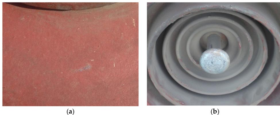
**Figure 8.** The contaminated insulator. (a) The upper surface; (b) The lower surface.
