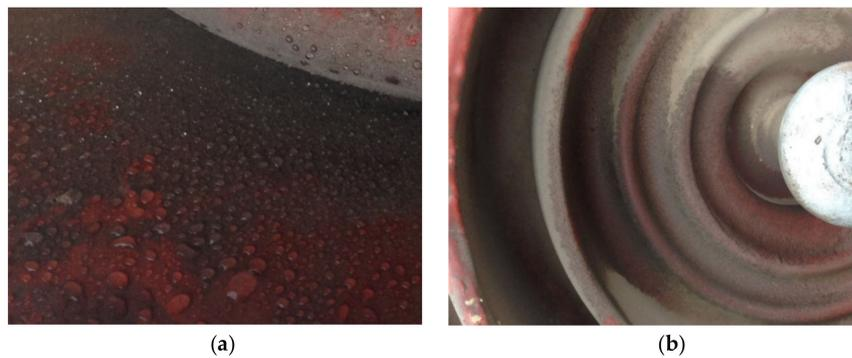
Figure 15. The hydrophobicity of the suspension insulator. (a) The upper surface; (b) the lower surface.
