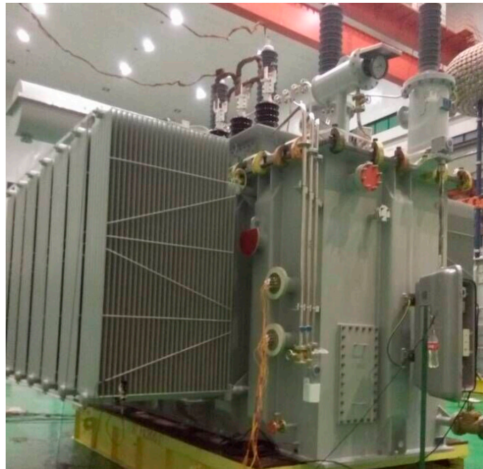
Figure 2. 110 kV three-phase three-limb transformer.
