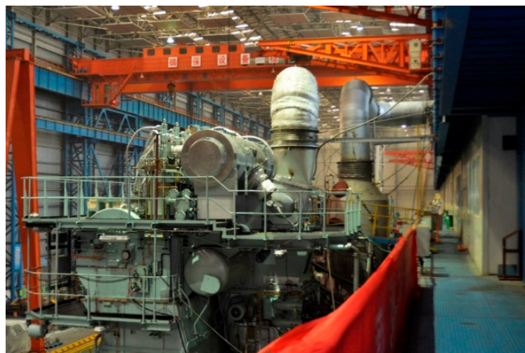
Figure 2. Photograph of the experimental setup for the scrubber in a marine diesel engine.
