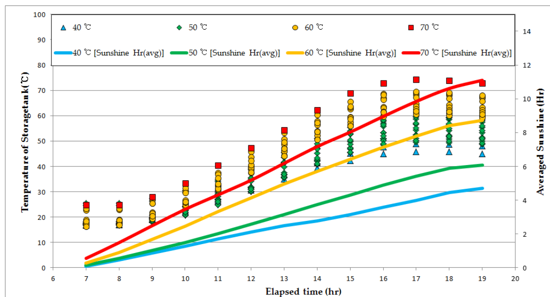
Figure 3. Temperature distribution of the heat storage tank and accumulated sunshine hours (11 April–6 May, 7:00 a.m.–7:00 p.m.).
