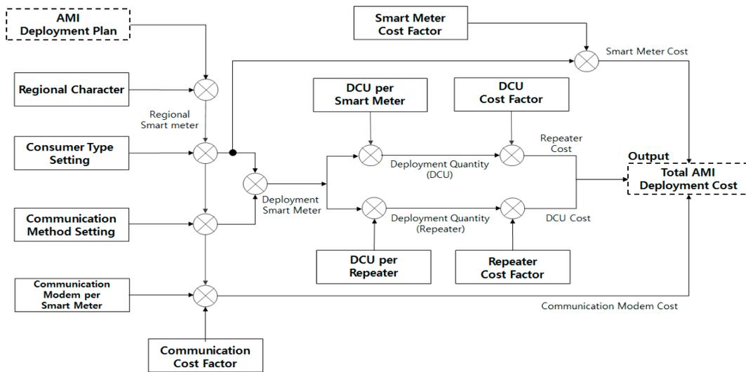
Figure 2. Hybrid AMI System Model.
