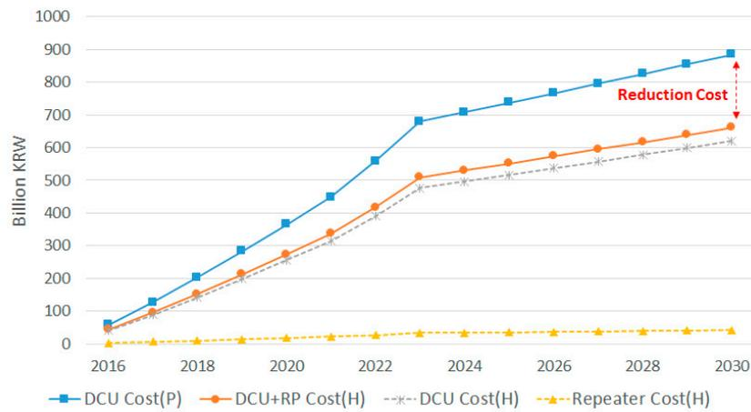
**Figure 7.** Comparison of DCU and Repeater Cost Results per Deployment Method (P: PLC-Only, H: Hybrid).
