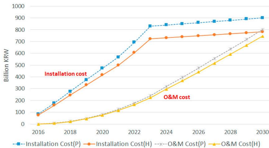
**Figure 6.** Comparison of Installation and O&M Cost Results per Deployment Method (P: PLC-Only, H: Hybrid).
