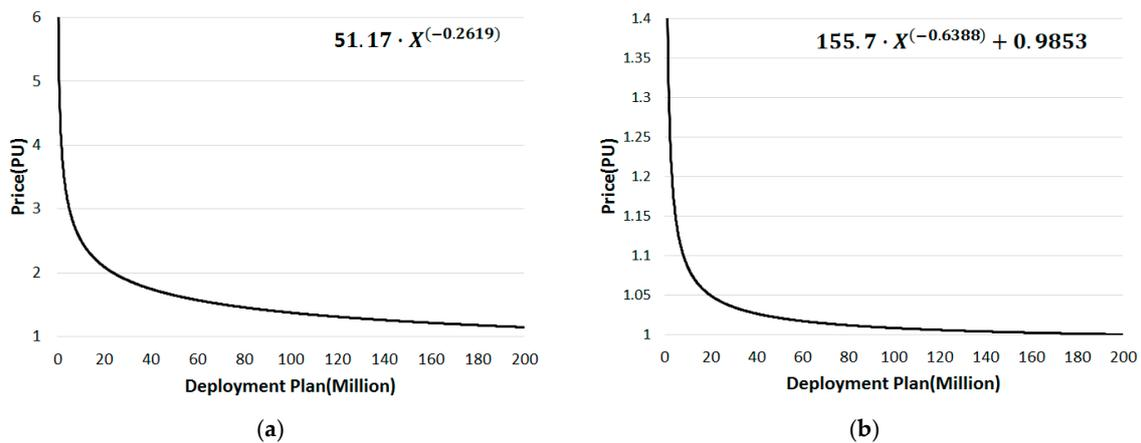
**Figure 4.** Communications Modem and DCU Cost Curve: (a) Communications Modem Cost Curve; (b) DCU Cost Curve.
