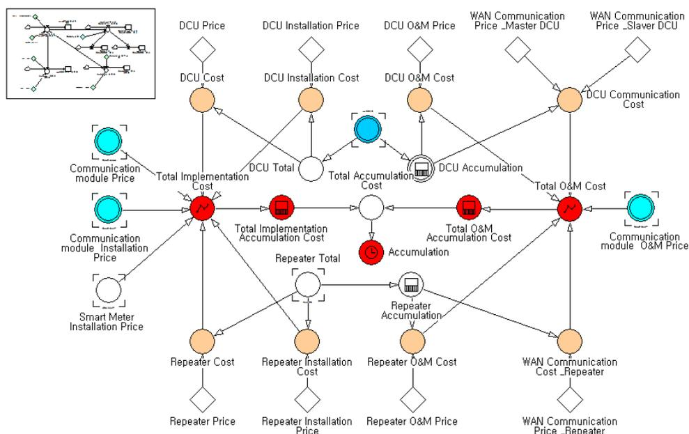
Figure 3. System Dynamics Modeling for Hybrid AMI.
