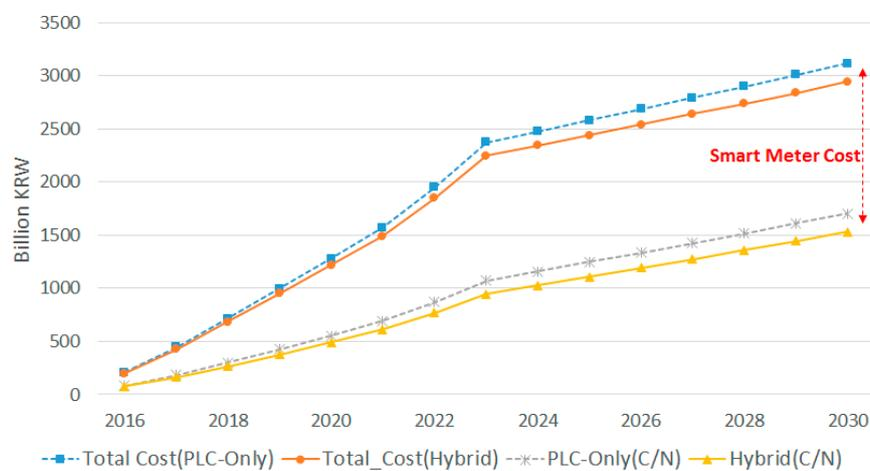
**Figure 5.** Costs by Deployment Type and Installation Item (C/N: Communication Networks).
