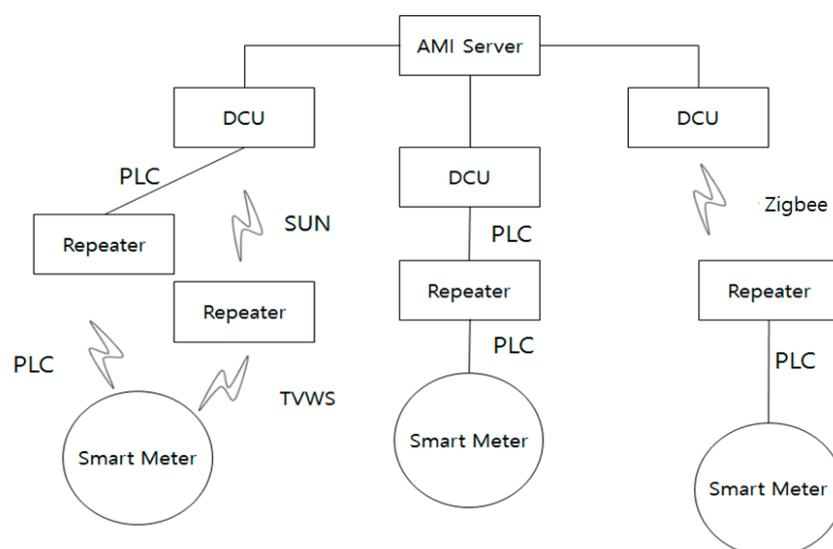
**Figure 1.** Hybrid Advanced Metering Infrastructure Structure.
