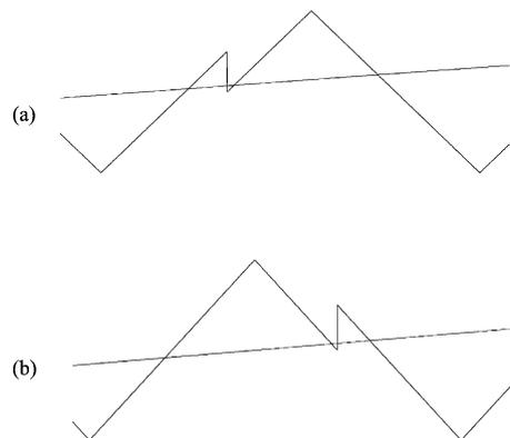
**Figure 2.** Illustration of the cases that the reference crosses the carrier four times in a cycle of the carries after a negative phase shift of the carriers: (a) Positive phase shift; (b) Negative phase shift.
