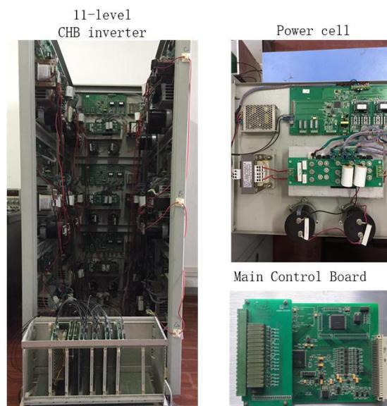
**Figure 14.** Picture of the experimental prototype.
