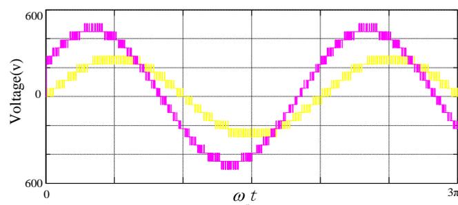
Figure 12. Phase and line voltage under the discontinuous modulation.
