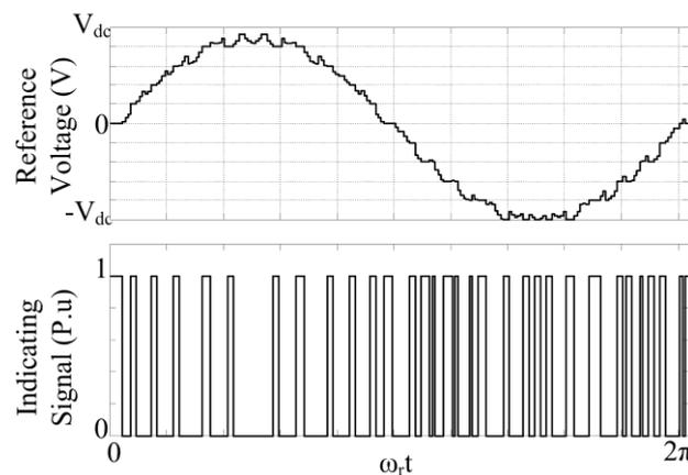
Figure 11. Reference and indicating signal under the discontinuous modulation.
