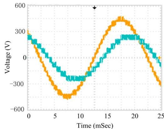
**Figure 15.** Experimental phase voltage and line voltage under the optimized new strategy (Modulation depth,  $M = 0.95$ ).
