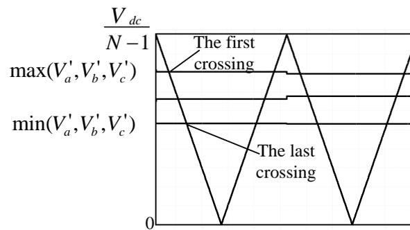
**Figure 5.** The common carrier and the new references  $V'_a$ ,  $V'_b$  and  $V'_c$ .
