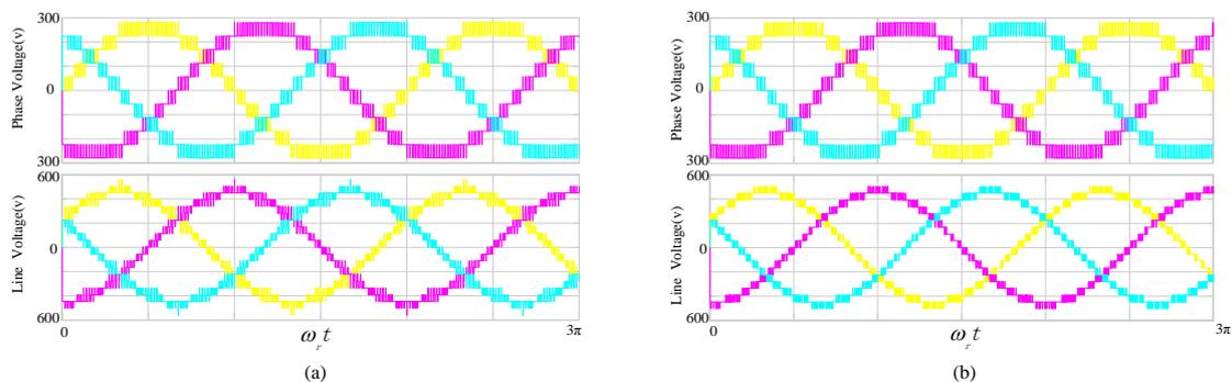
**Figure 7.** Phase voltage and line voltage for PS-PWM and the optimized new strategy: (a) Phase voltage and line voltage for PS-PWM; (b) Phase voltage and line voltage for the optimized new strategy.
