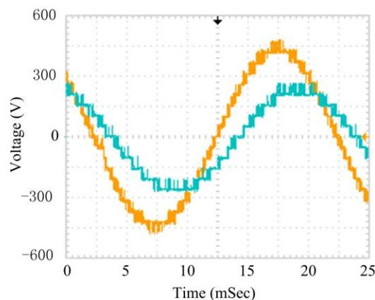
**Figure 16.** Experimental phase voltage and line voltage under discontinuous modulation strategy (Modulation depth,  $M = 0.95$ ).
