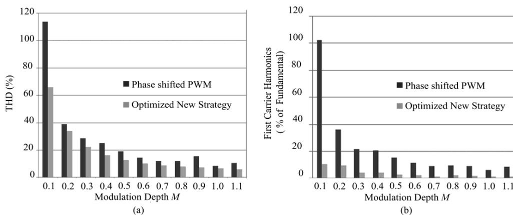
**Figure 9.** Detailed comparison of the THD and first carrier harmonics about the line voltage PS-PWM and the optimized new strategy: (a) Comparison of THD; (b) Comparison of first carrier harmonics.
