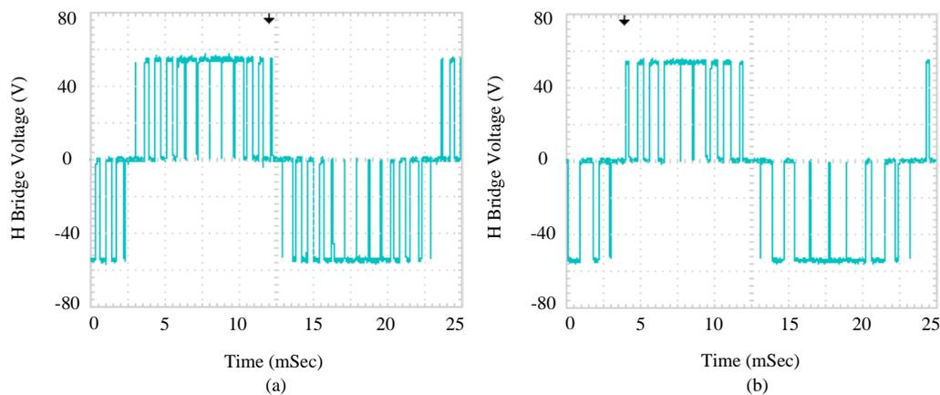
**Figure 17.** Output voltages of one power cell under the optimized new strategy and discontinuous modulation strategy (Modulation depth,  $M = 0.95$ ): (a) Output voltage under the optimized new strategy; (b) Output voltage under discontinuous modulation strategy.
