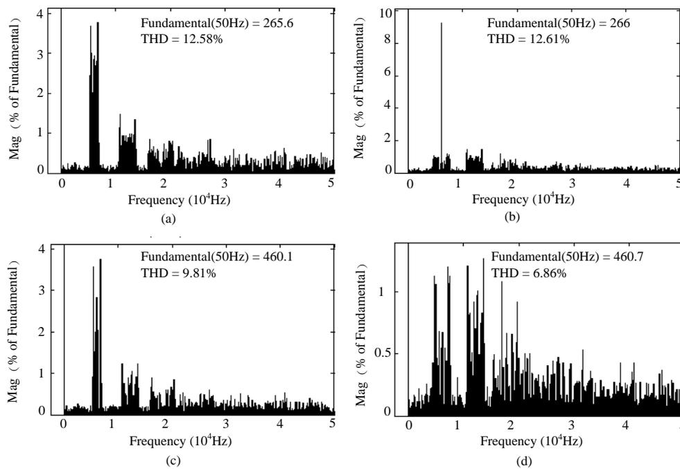
**Figure 8.** Spectrum of phase voltage and line voltage for PS-PWM and the optimized new strategy (Modulation depth,  $M = 0.95$ ): (a) Spectrum of phase voltage for PS-PWM; (b) Spectrum of phase voltage for the optimized new strategy; (c) Spectrum of line voltage for PS-PWM; (d) Spectrum of line voltage for the optimized new strategy.
