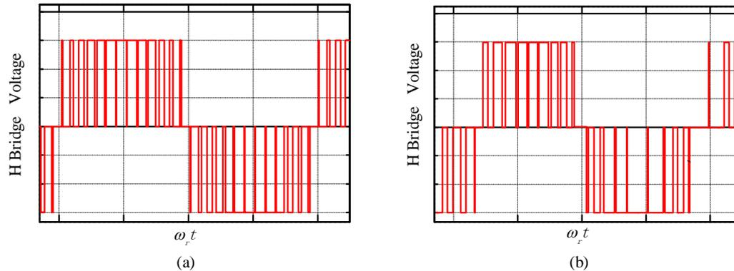
**Figure 13.** The output voltage of the power cell under continuous modulation and discontinuous modulation. (a) Output voltage under continuous modulation; (b) Output voltage under discontinuous modulation.
