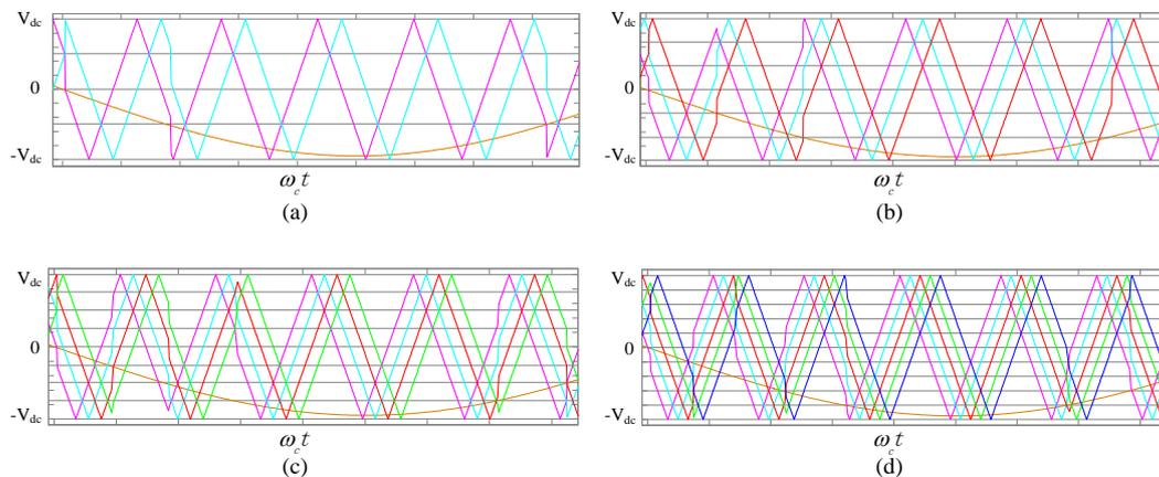
**Figure 6.** Carriers and reference under the optimized new strategy under CHB inverters of various levels. (a) New strategy for five-level CHB inverter; (b) New strategy for seven-level CHB inverter; (c) New strategy for nine-level CHB inverter; (d) New strategy for 11-level CHB inverter.
