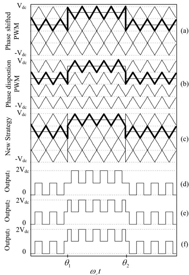
**Figure 1.** Modulation strategies and the corresponding output voltages: (a) phase-shifted pulse width modulation (PS-PWM) and phase disposition pulse width modulation (PS-PWM); (b) PD-PWM; (c) New strategy; (d) Output voltage for PS-PWM; (e) Output voltage for PD-PWM; (f) Output voltage for new strategy.
