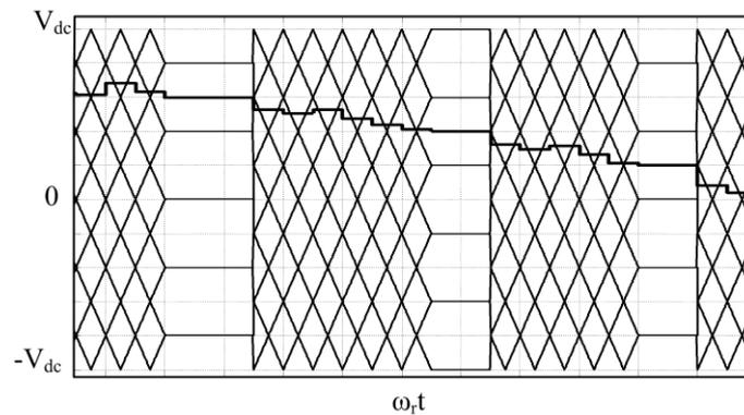
Figure 10. Carriers and reference under the discontinuous modulation.
