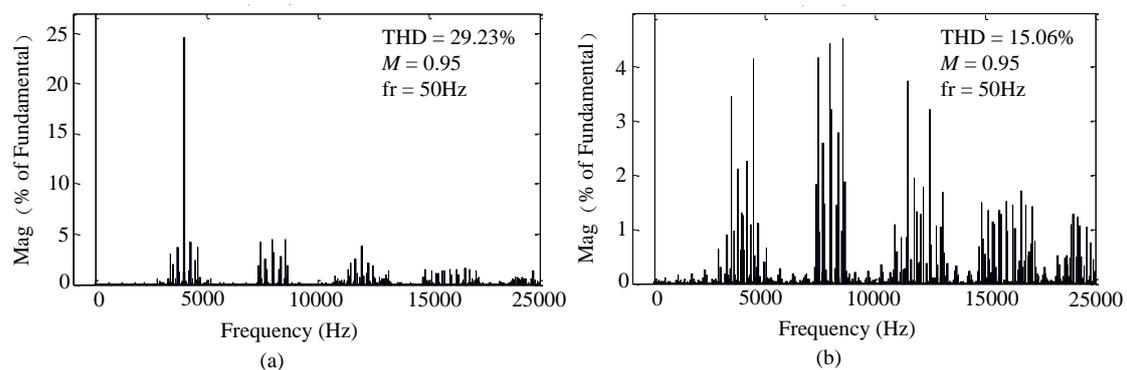
**Figure 4.** The spectrum of line voltage for a five-level cascaded H-bridge (CHB) inverter under different condition. Switching frequency is 1 kHz. Modulation depth,  $M = 0.95$ . Reference frequency is 50 Hz: (a) Harmonics profile of line voltage where the equivalent carriers for phase A and B are opposite in phase; (b) Harmonics profile of line voltage where the equivalent carriers for phase A and B are in phase.
