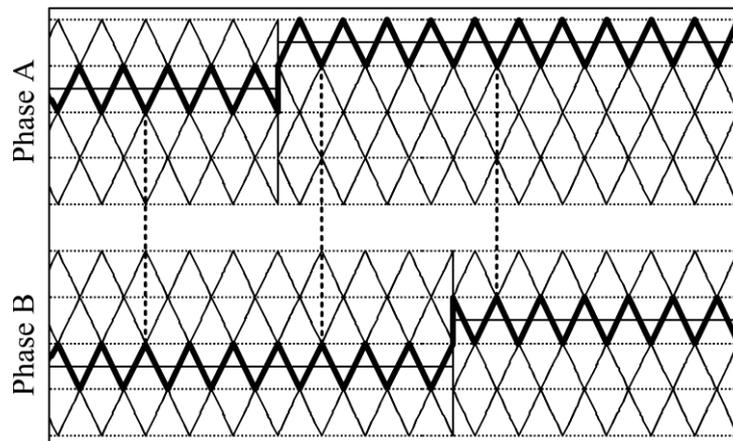
**Figure 3.** Phase deviation of equivalent carriers between (phase A, B) caused by the different initial position of references.
