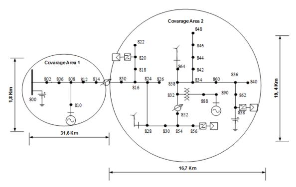
Figure 1. Modified distribution system model with distributed energy resources.
