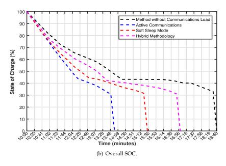
**Figure 2.** (a) comparison of power consumption for several methodologies; (b) comparison of state of charge for several methodologies.
