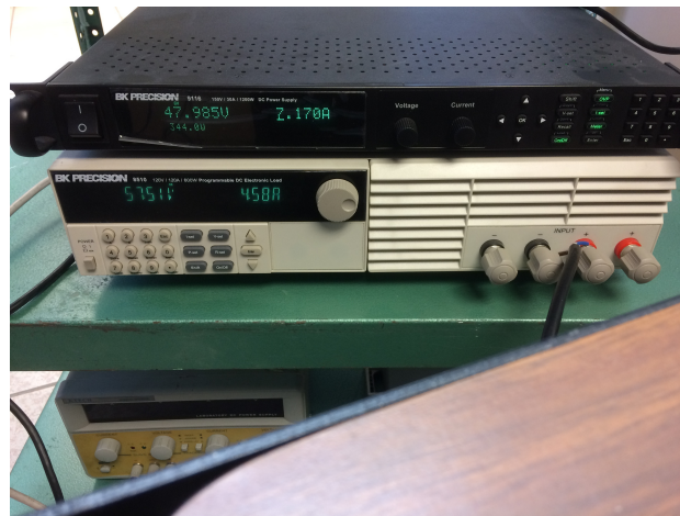
Figure 16. Main power supply and electronic load in Mode II with 3 \Omega load.
