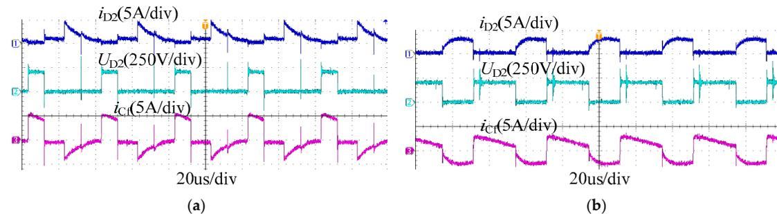
**Figure 20.** Tested voltage and current waveforms of  $D_2$  and current waveform of  $C_1$ : (a)  $U_{in} = 48$  V; (b)  $U_{in} = 120$  V.
