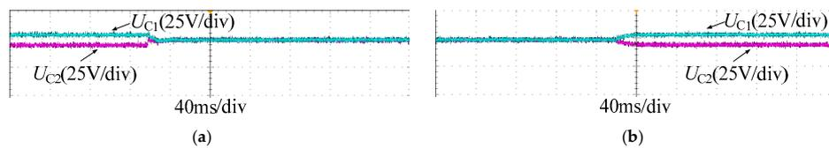
**Figure 23.** Voltage balance process of  $C_1$ ,  $C_2$  when  $U_{in}$  is 120 V: (a) from no voltage-balance control to voltage-balance control; (b) from voltage-balance control to no voltage-balance control.
