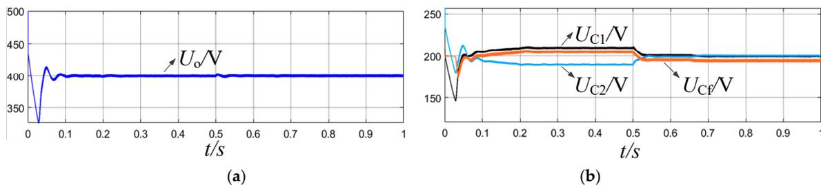
**Figure 11.** Simulated voltage waveforms when  $U_{in}$  is 48 V: (a)  $U_o$ ; (b)  $U_{C1}$ ,  $U_{C2}$ , and  $U_{Cf}$ .
