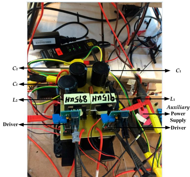
**Figure 15.** The experimental prototype.
