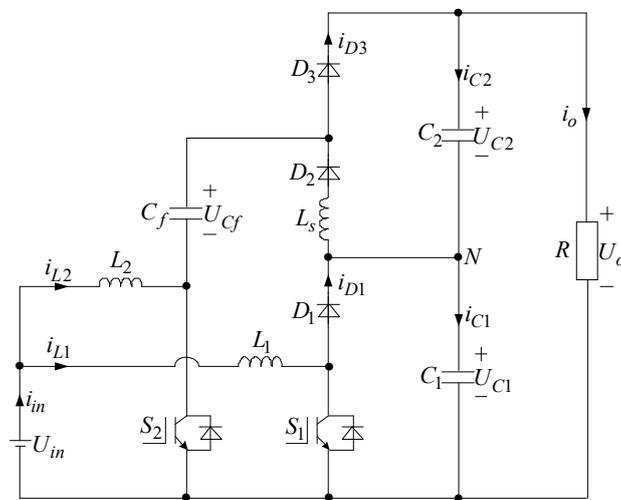
Figure 8. IPOS-SC-TLB with a small stray inductor  $L_s$ .
