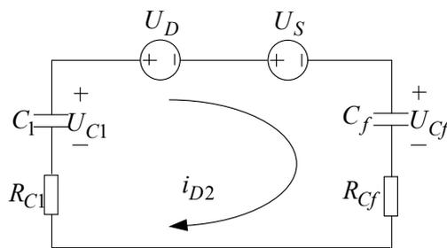
Figure 7. Equivalent circuit of the switched-capacitor network.
