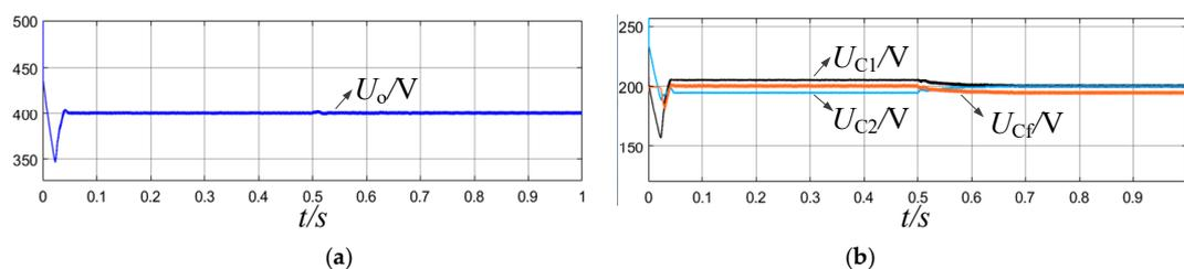
**Figure 12.** Simulated voltage waveforms when  $U_{in}$  is 120 V: (a)  $U_o$ ; (b)  $U_{C1}$ ,  $U_{C2}$ , and  $U_{Cf}$ .
