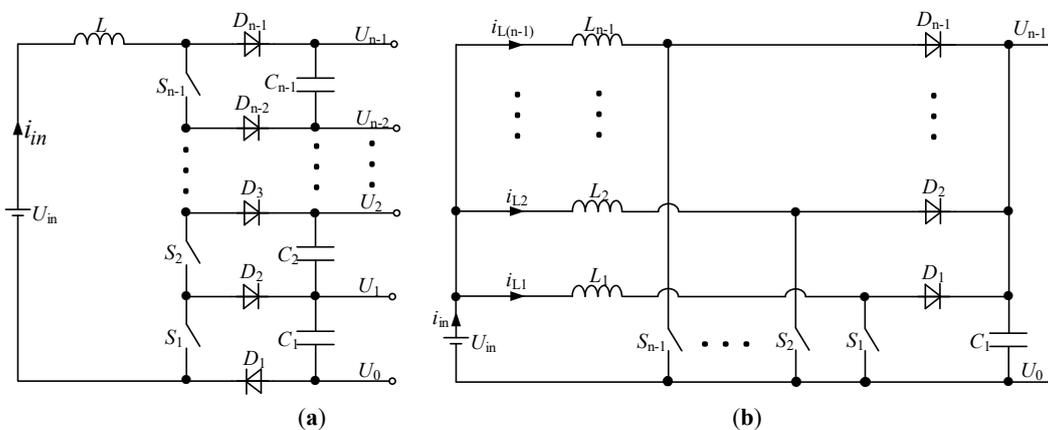
Figure 1. Two interleaved structures: (a) SI; (b) PI.
