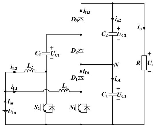
Figure 3. The proposed IPOS-SC-TLB converter.
