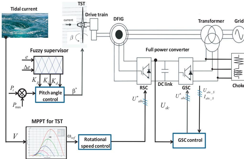
**Figure 4.** Tidal stream generator control scheme. TST , Doubly Fed Induction Generator (DFIG), Rotor Side Converter (RSC), Grid Side Converter (GSC), Maximum Power Point Tracking (MPPT).
