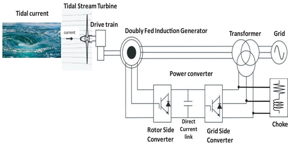
**Figure 2.** Scheme of the tidal stream generator system [30].
