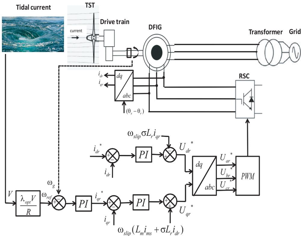
Figure 12. RSC control scheme design.
