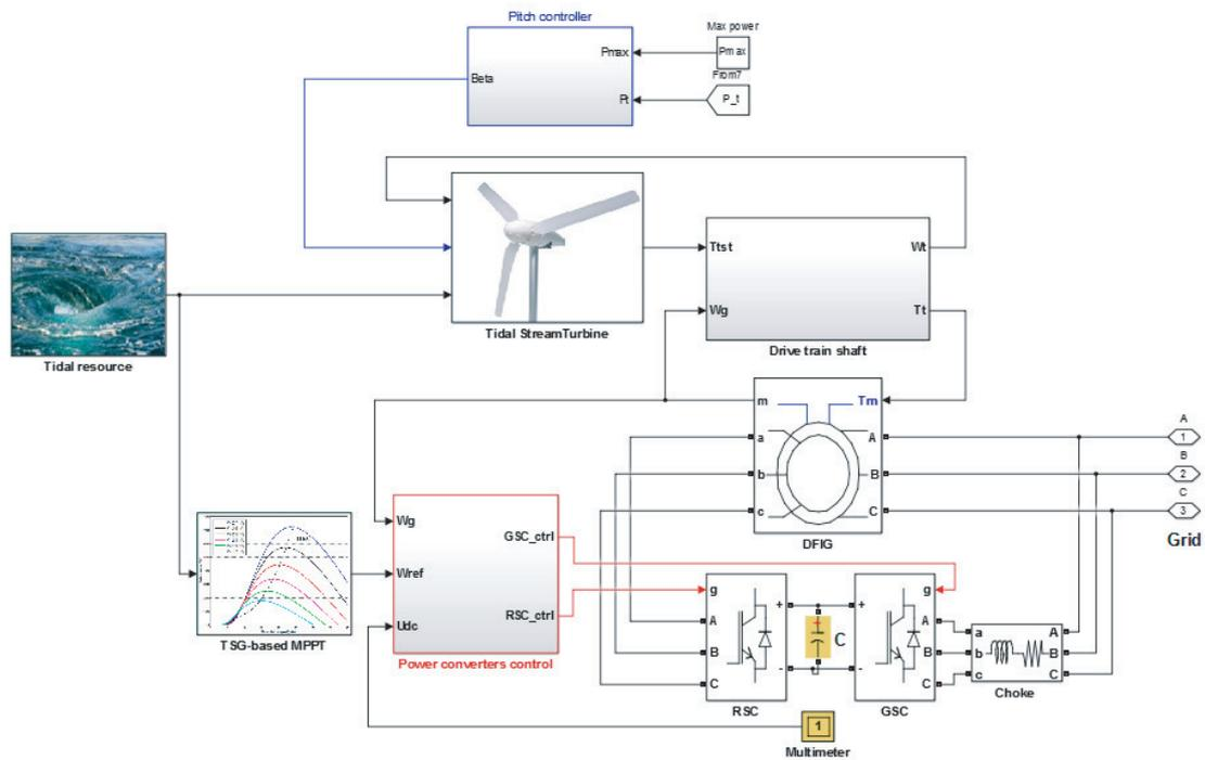
**Figure 15.** Model implementation of the TSG power plant.
