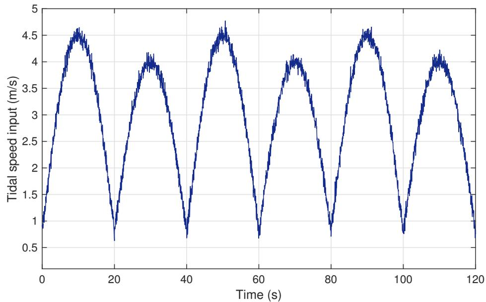
**Figure 16.** Case 1: Regular turbulent tidal resource speed.
