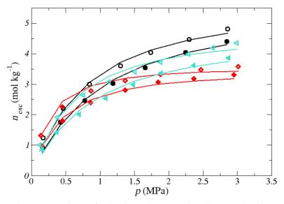
**Figure 2.** CH<sub>4</sub> adsorption isotherms for the three olive stone-based activated carbons: AC-H<sub>3</sub>PO<sub>4</sub> (black circles), AC-CO<sub>2</sub> (red diamonds) and AC-H<sub>2</sub>O (turquoise triangles). Open symbols represent the adsorption data at 303.15 K, while the data at 323.15 are shown by the filled symbols. Uncertainties:  $\Delta p = 0.01$  MPa,  $\Delta T = 0.2$  K. The obtained Langmuir fitting isotherms are shown by the solid lines.
