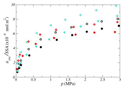
**Figure 4.** SSA normalized  $CO_2$  adsorption isotherms of the activated carbons:  $AC-H_3PO_4$  (black circles),  $AC-CO_2$  (red diamonds) and  $AC-H_2O$  (turquoise triangles). Open symbols represent the adsorption data at 303.15 K, while the data at 323.15 are shown by the filled symbols 323.15 K.
