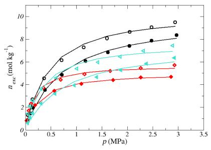
**Figure 3.** CO<sub>2</sub> adsorption isotherms for the three olive stone-based activated carbons: AC-H<sub>3</sub>PO<sub>4</sub> (black circles), AC-CO<sub>2</sub> (red diamonds) and AC-H<sub>2</sub>O (turquoise triangles). Open symbols represent the adsorption data at 303.15 K, while the data at 323.15 are shown by the filled symbols. Uncertainties:  $\Delta p = 0.01$  MPa,  $\Delta T = 0.2$  K. The obtained Langmuir fitting isotherms are shown by the solid lines.
