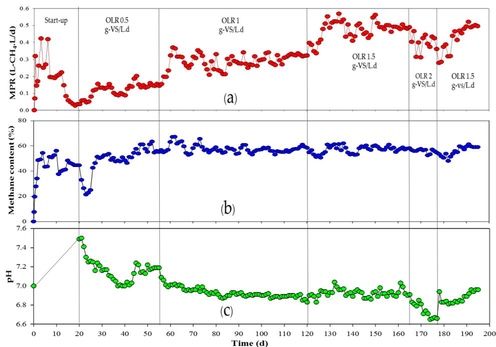
**Figure 1.** Effect of organic loading rate (OLR) on the performance of a horizontal reactor. (a) methane production rate (MPR), (b) methane content and (c) pH.
