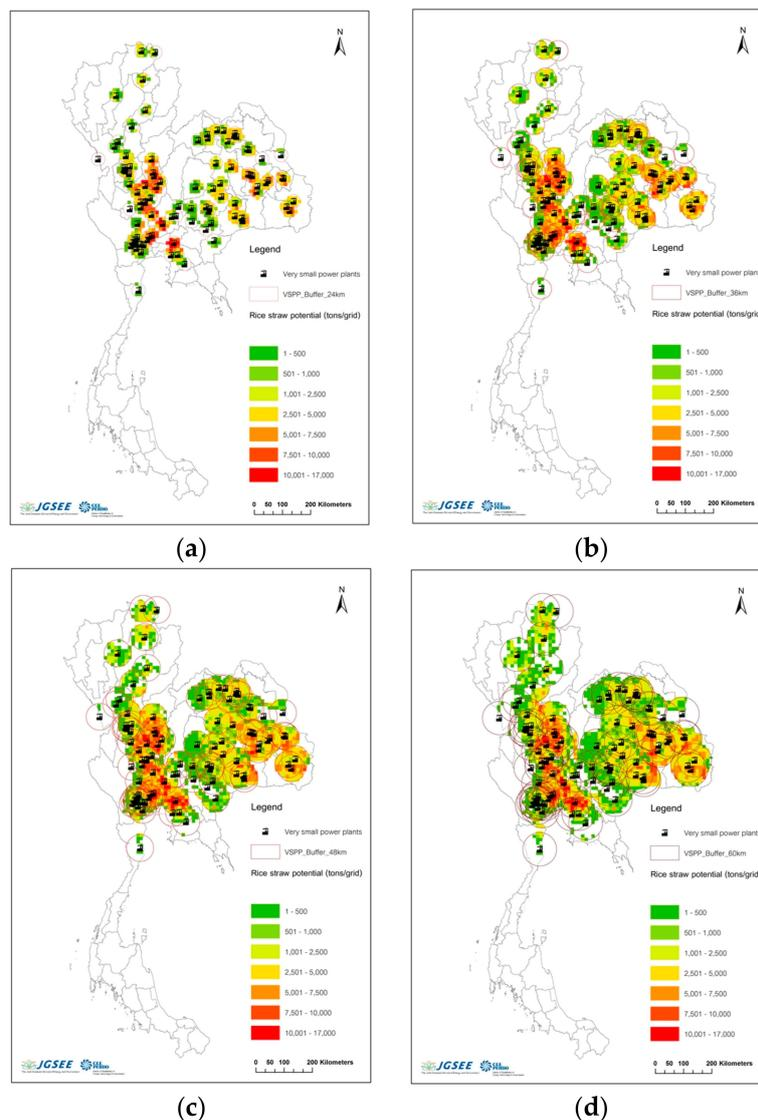
**Figure 13.** Efficiency of supply fuel for very small biomass power plants at various radii: (a) 24 km, (b) 36 km, (c) 48 km, and (d) 60 km.
