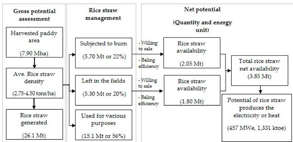
Figure 12. Material flow diagram of rice straw residue for energy-related purposes.
