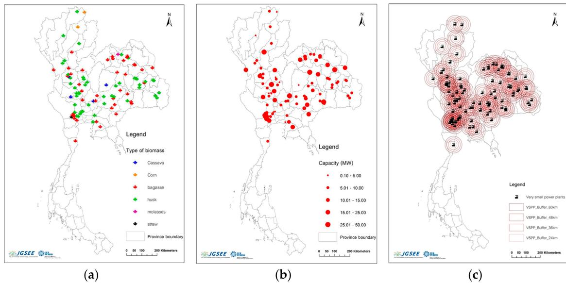
**Figure 6.** Very small biomass power plants categorized by (a) type of biomass fuel, and (b) capacity of very small power plants (VSPPs); (c) the radii of collected rice straw residue.
