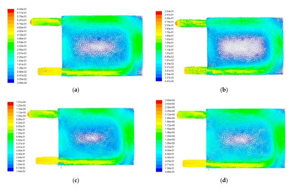
Figure 8. Velocity vectors of structure B. (a) v = 0.2 m/s; (b) v = 0.5 m/s; (c) v = 1.0 m/s; (d) v = 2.0 m/s.
