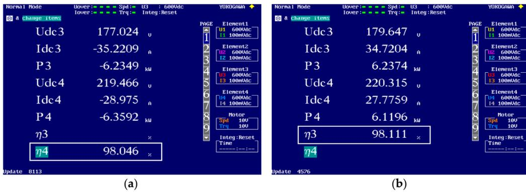
Figure 14. Efficiency of four-leg converter: (a) Charge mode; (b) Discharge mode.
