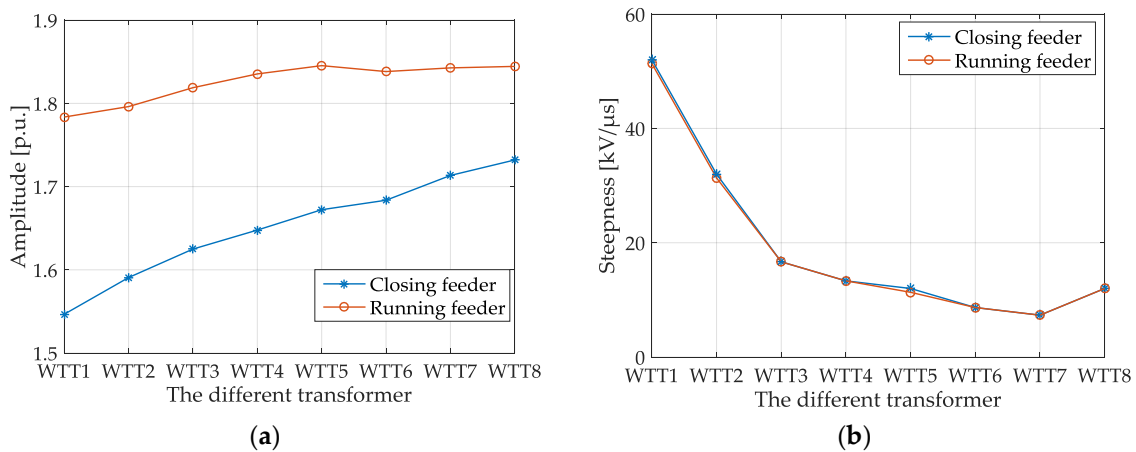
Figure 11. The overvoltage of different transformer locations for Scenario 3: (a) amplitude; (b) steepness.
