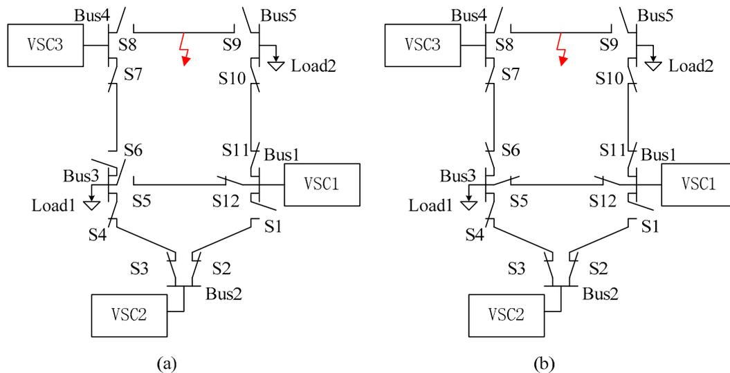
**Figure 10.** Switch operations of the improved handshaking method: (a) Switches state after step 2; (b) Switches state after step 4.
