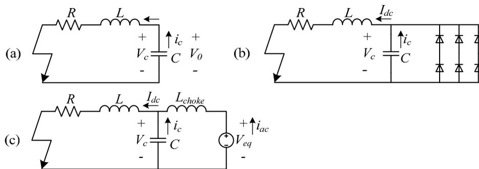
**Figure 1.** The equivalent circuits of different stages: (a) Stage 1: Capacitor discharge; (b) Stage 2: Diodes freewheel; and (c) Stage 3: Grid current feeding.
