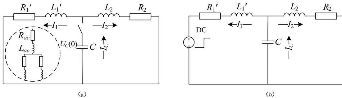
**Figure 5.** The equivalent transient-state circuit model of VSC: (a) the natural response process equivalent circuit; and (b) the forced response process equivalent circuit.
