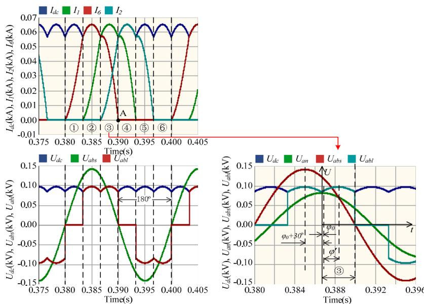
Figure 4. The waveform of steady-state quantities in Figure 3:  $I_{dc}$ ,  $I_1$ ,  $I_2$ , and  $I_6$  (in kA);  $U_{dc}$ ,  $U_{abl}$ ,  $U_{abs}$  and  $U_{an}$  (in kV).
