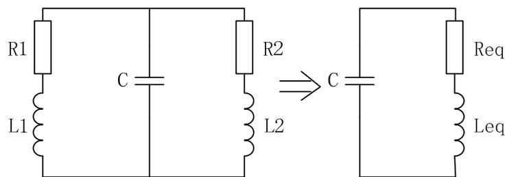
Figure 6. The equivalent convert of the RLC circuit.
