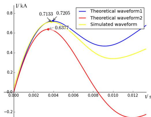
**Figure 7.** The waveform of the surge current of simulated values; theoretical values in [4] and this paper.
