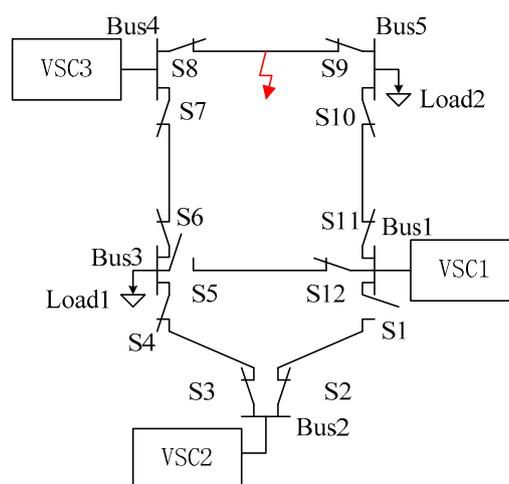
**Figure 8.** The structure of a multi-terminal loop-type DC distribution network.
