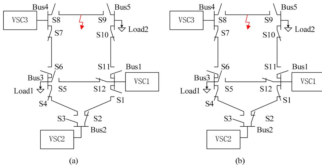
**Figure 9.** Switch operations of the classical handshaking method: (a) Switches state after step 2; (b) Switches state after step 4.
