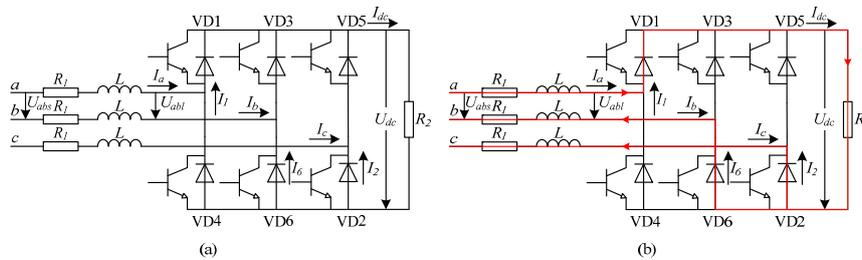
Figure 3. The equivalent circuit for analysis: (a) The simplified circuit model of VSC; (b) The current path and direction.
