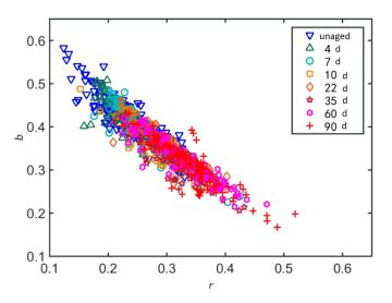
Figure 5. r, b values of chromatic dispersion images for fibers under different aging stages.
