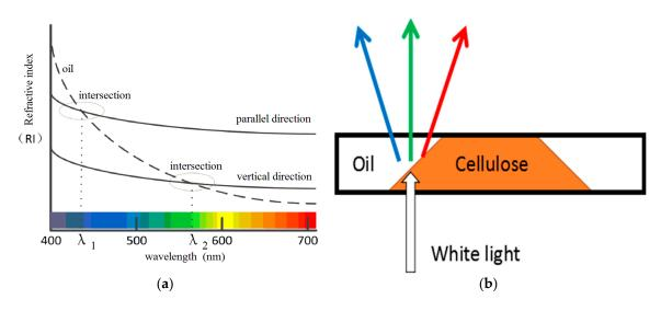
Figure 1. (a) Matching wavelength diagram; (b) dispersion of fiber.
