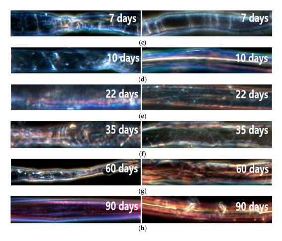
**Figure 4.** Typical chromatic dispersion color of fibers in oil at different aging stages. (**a**) 0 days for aging; (**b**) 4 days for aging; (**c**) 7 days for aging; (**d**) 10 days for aging; (**e**) 22 days for aging; (**f**) 35 days for aging; (**g**) 60 days for aging; (**h**) 90 days for aging.
