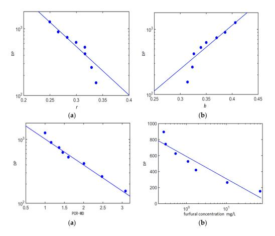
**Figure 6.** (a) Fitting of DP and r; (b) Fitting of DP and b; (c) Fitting of DP and D; (d) Fitting of DP and furfural concentration.
