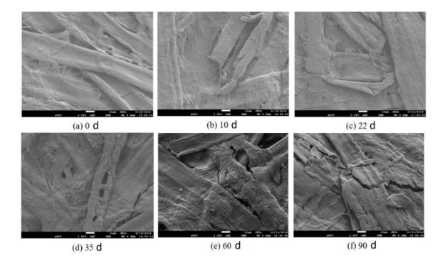
Figure 3. Fiber morphology at different aging times.
