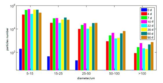
Figure 2. Particle size distribution of fibers in oil with different aging days at 130 °C.
