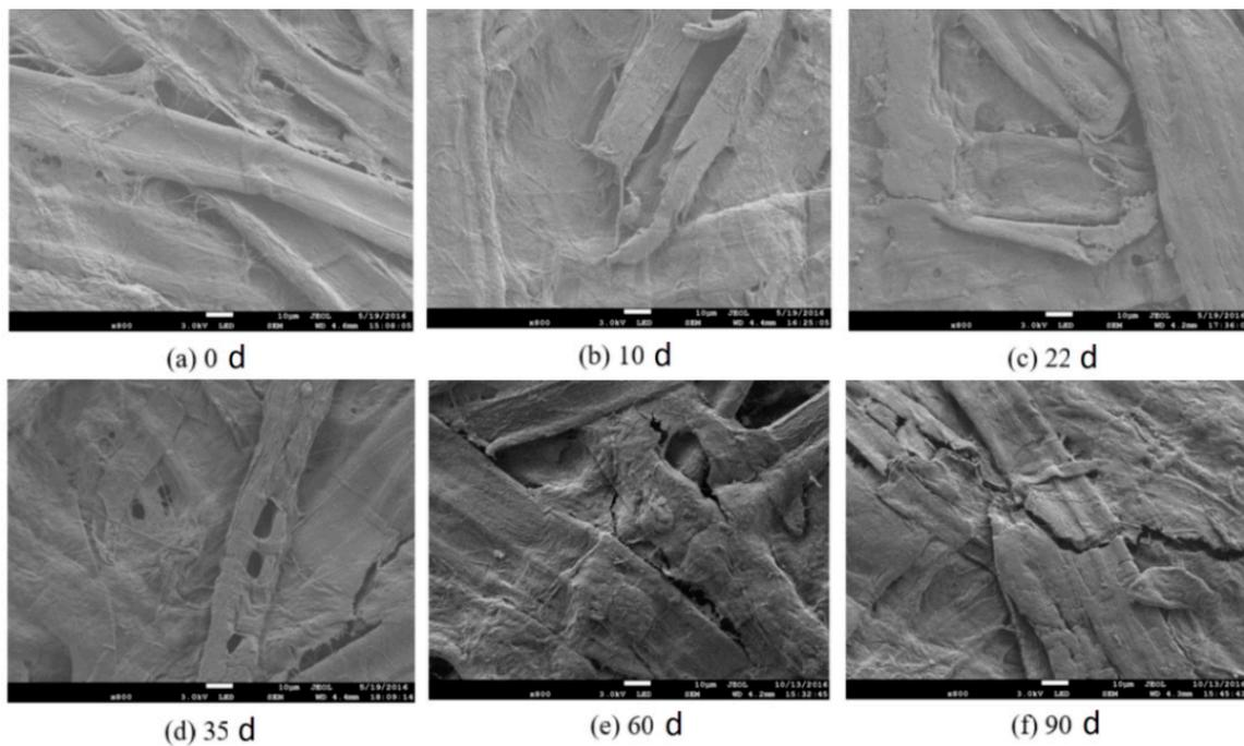
**Figure 3.** Fiber morphology at different aging times.
