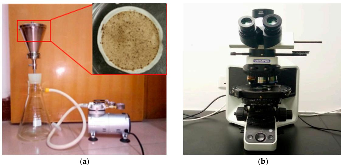
**Figure 7.** (a) Experimental filter device; (b) polarizing microscope.
