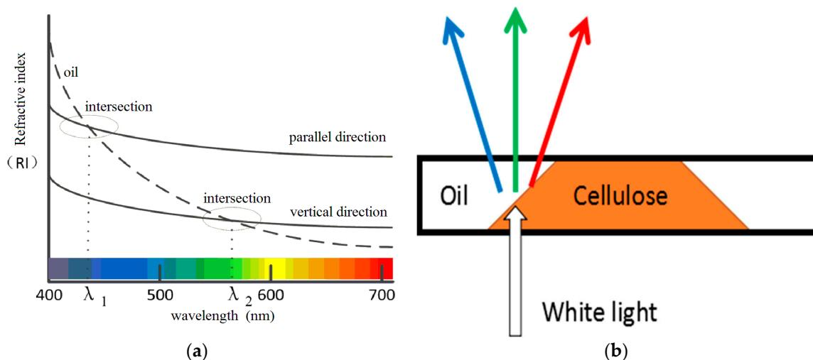
**Figure 1.** (a) Matching wavelength diagram; (b) dispersion of fiber.
