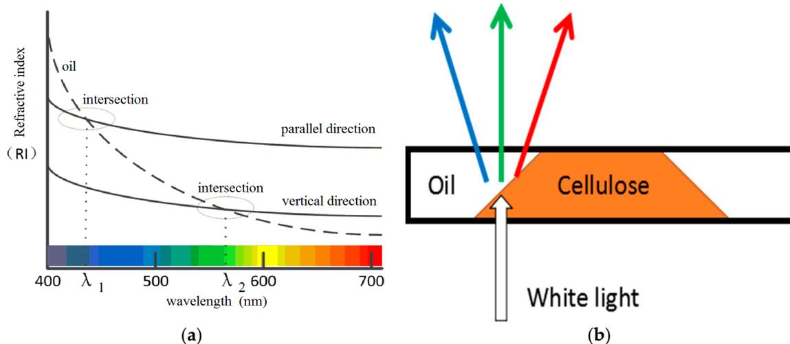
**Figure 1.** (a) Matching wavelength diagram; (b) dispersion of fiber.
