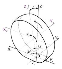
Figure 4. Tyre with camber angle.
