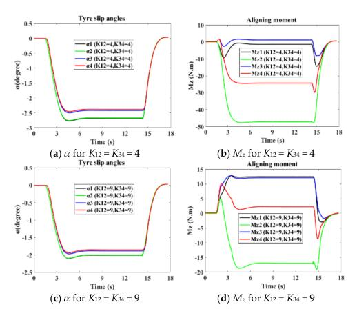
**Figure 13.** Slip angle and aligning moment at R = 100 m and  $V_x = 88.18$  km/h.
