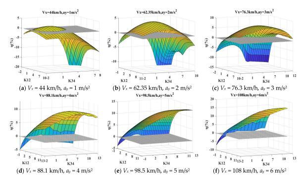
**Figure 16.** Energy saving for different  $K_{12}$  and  $K_{34}$  for path R = 150 m and L = 90 m.
