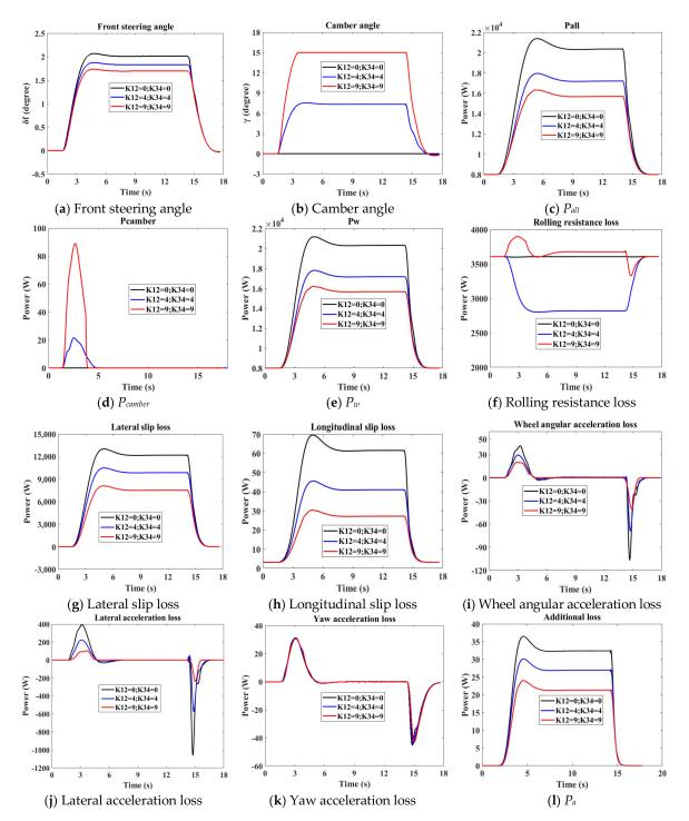
to be comparatively large. Consequently, further increasing the camber angle,  $\sum_{i=1}^{4} M_{zi} \sin \gamma_i$  does not increase much and the reduction of lateral slip loss still plays a dominant role in energy saving.
