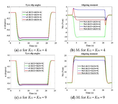
**Figure 12.** Slip angle and aligning moment at R = 100 m and  $V_x = 62.3$  km/h.
