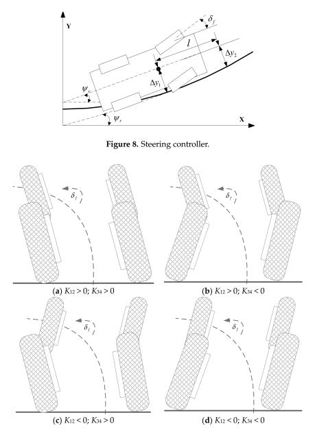
Figure 9. Rear views of the vehicle with different settings on camber control coefficient  $K_{12}$  and  $K_{34}$ .
