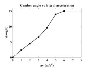
Figure 17. Camber control versus lateral acceleration.
