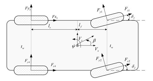
Figure 5. Two-track vehicle model.
