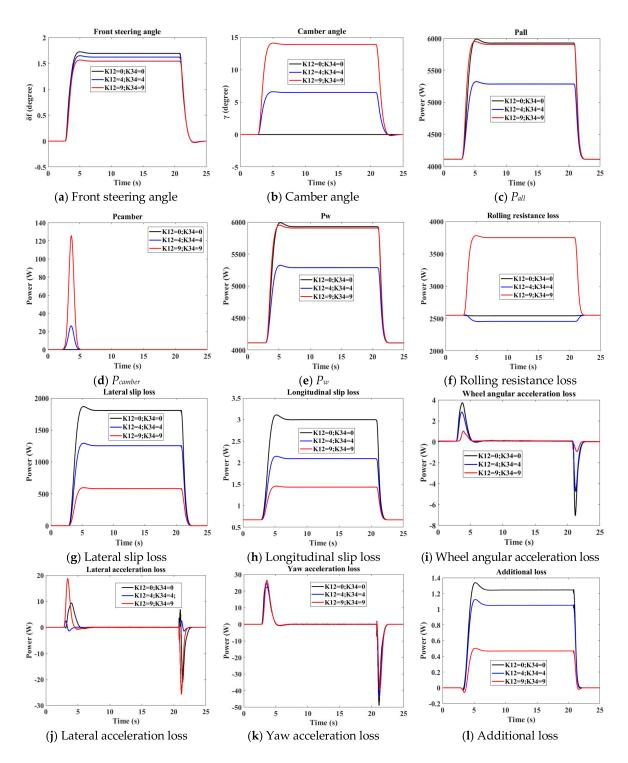
**Figure 10.** Steering and camber angles as well as power losses at R = 100 m and  $V_x = 62.3$  km/h.
