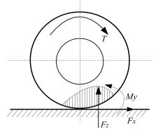
Figure 3. Tyre without camber angle.
