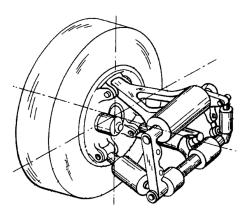
Figure 1. Active wheel corner module [8].
