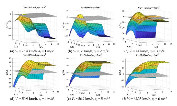
**Figure 14.** Energy saving for different  $K_{12}$  and  $K_{34}$  for path R = 50 m and L = 30 m.
