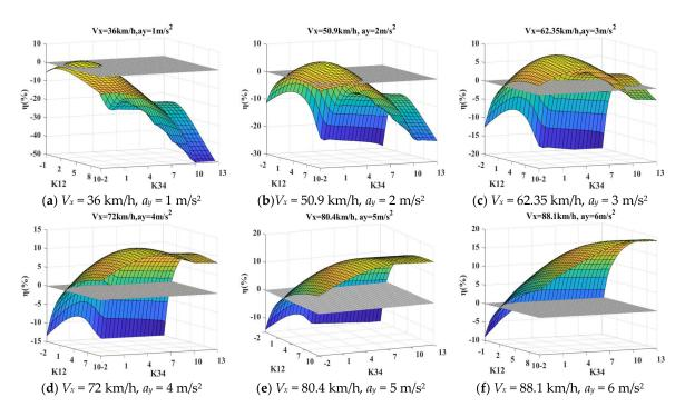
**Figure 15.** Energy saving for different  $K_{12}$  and  $K_{34}$  for path R = 100 m and L = 60 m.
