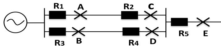
Figure 6. A single end fed parallel feeder distribution system.
