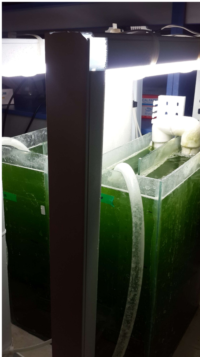
Figure 5. Raceway pond and airlift pump (RWPAP) reactor.
