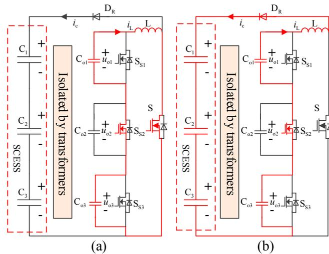
Figure 5. The currents of the boost converter. (a) The switch S is turned on; (b) The switch S is turned off.
