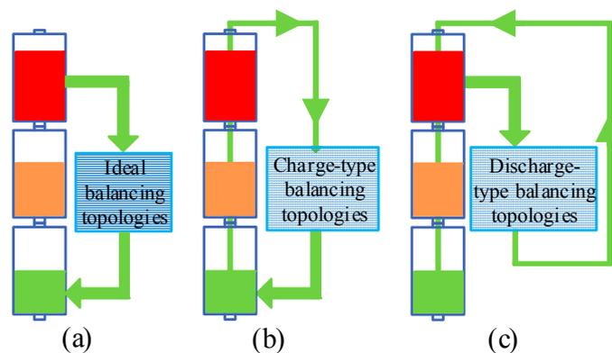
**Figure 1.** Classification of balancing system based on the ways that energy can be transferred. (a) With ideal balancing topologies; (b) With charge-type balancing topologies; (c) With discharge-type balancing topologies.
