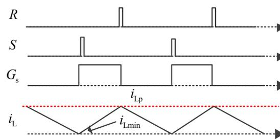
Figure 14. The main waveforms of the boost converter.
