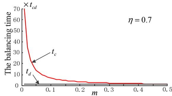
Figure 18. The balancing time  $t_c(t_d)$  change with charge (discharge) number  $m$ .
