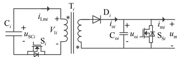
Figure 6. The cascaded converter module.
