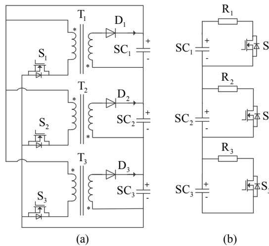
**Figure 24.** Charge and discharge type balancing topology used in the comparative experiment. (a) Charge type in [18]. (b) Discharge type in [22].
