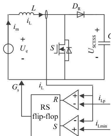
**Figure 13.** Control circuit diagram of the boost converter with hysteresis current control strategy.
