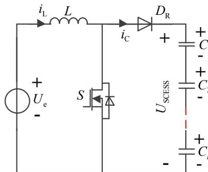
Figure 8. The simplified boost converter.
