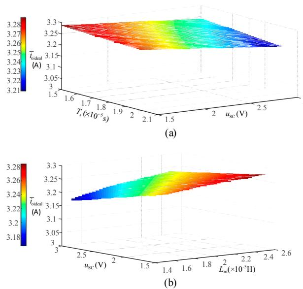
**Figure 12.** Ideal output current varies with  $u_{sc}$ ,  $T_s$ , and  $L_m$ . (a) Ideal output current varies with  $u_{sc}$  and  $T_s$ . (b) Ideal output current varies with  $u_{sc}$  and  $L_m$ .
