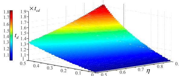
Figure 17. The balancing time of discharge-type topology  $t_d$  changing with  $m_2$ ,  $\eta$ .
