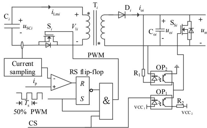
Figure 9. Control circuit of the cascaded converter module.
