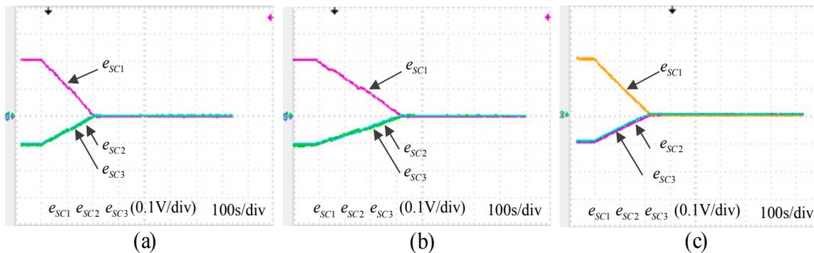
**Figure 25.** The balancing time of the comparative experiment. (a) Proposed modularized discharge-type topology. (b) Charge-type balancing topology. (c) Switched resistor method.
