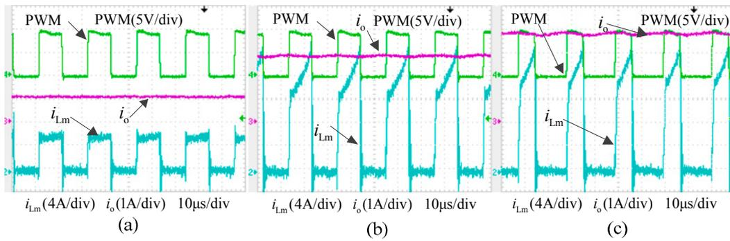
**Figure 20.** Main waveforms of the modularized converter module. (a) With output current  $i_o = 1$  A. (b) With output current  $i_o = 3.1$  A. (c) With output current  $i_o = 4$  A.
