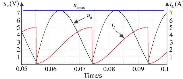
**Figure 15.** Waveform of  $u_o$  and  $i_L$  with the PWM frequency slightly higher than two times of the resonant frequency of  $L$  and  $C_o$ .
