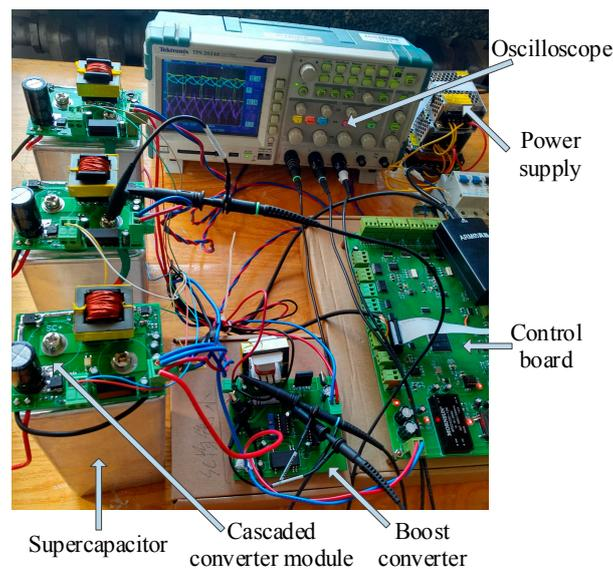
**Figure 19.** The photograph of the experiment platform.
