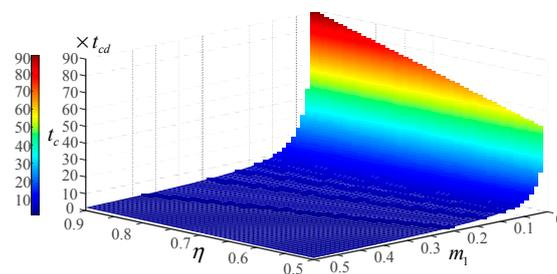
Figure 16. The balancing time of charge-type topology  $t_c$  changing with  $m_1$ ,  $\eta$ .
