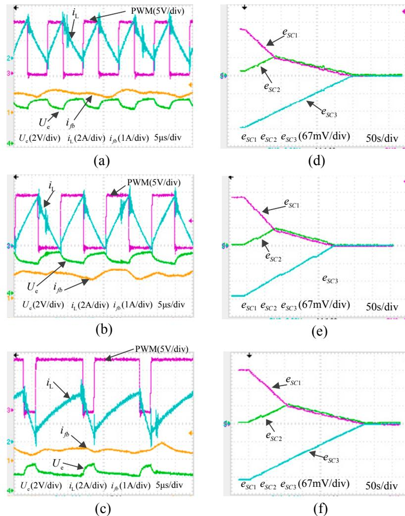
**Figure 23.** The main waveforms of the boost converter and the balancing time. (a)–(c) are the main waveforms of the boost converter with 2 A, 3.1 A, and 3.6 A average input current, respectively. (d)–(f) are the corresponding balancing time.
