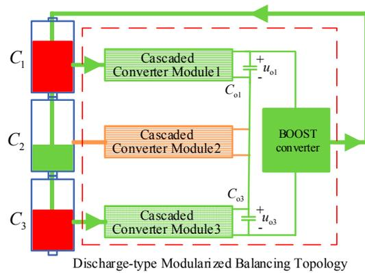
Figure 3. The balancing principle block diagram of the proposed topology.
