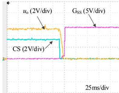
**Figure 22.** The drive of short circuit switch  $S_S$ .
