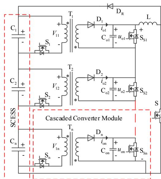
**Figure 2.** The proposed modularized discharge-type equalizer.
