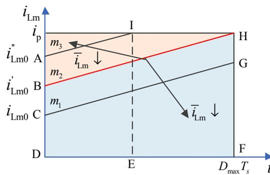
Figure 11. The current  $i_{Lm}$  changing with time.
