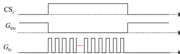
Figure 7. The drives of the cascaded converter module.
