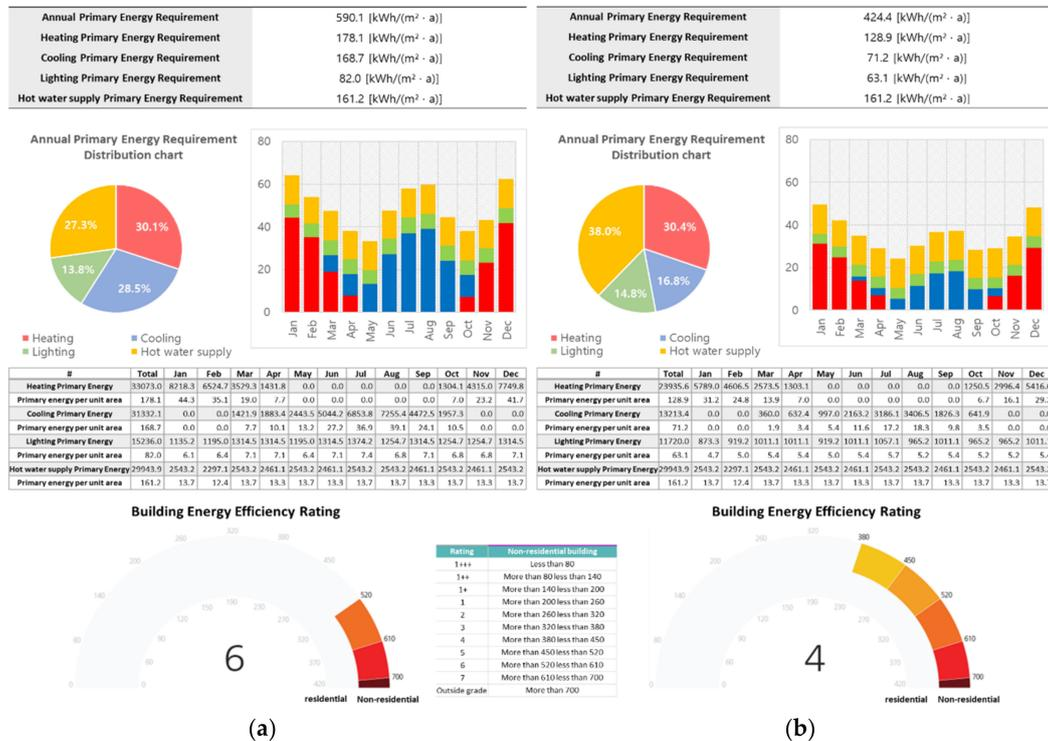
**Figure 9.** Estimated primary energy requirement and energy efficiency rate before and after providing the energy visualization solution (testbed 2). (a) Before application of visualization solution; (b) After application of visualization solution.
