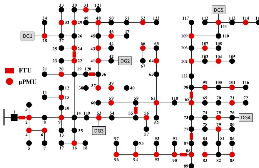
**Figure 6.** Optimal  $\mu$ PMU placement by improved IENS.
