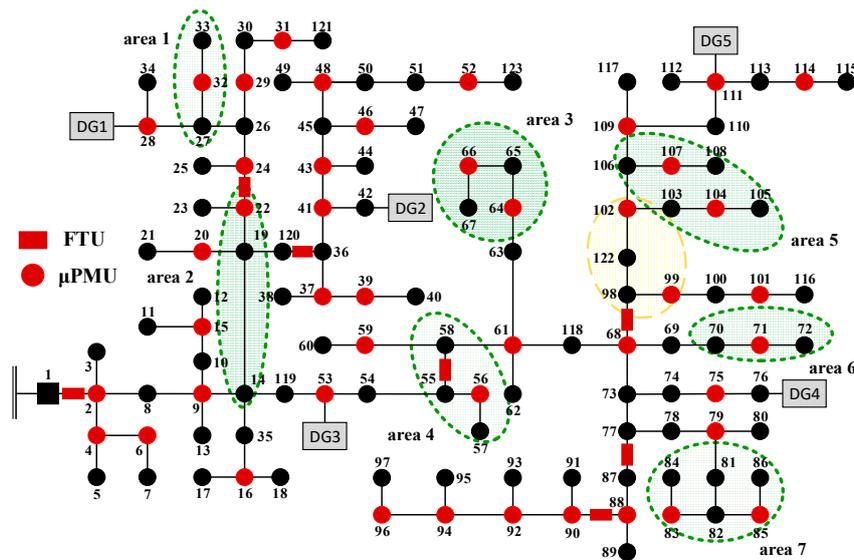
Figure 9. Optimal  $\mu$ PMU placement by improved IENS.
