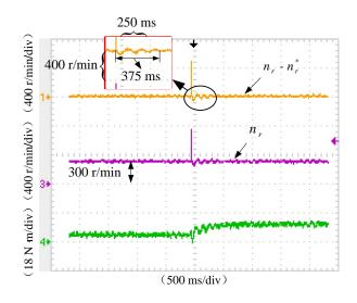
**Figure 22.** Experimental results of DTC (P = 20, I = 0.8).
