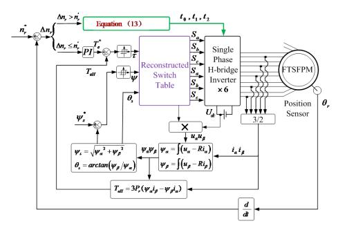
Figure 14. The RDTC system with torque integral balance control (TIBC-RDTC).
