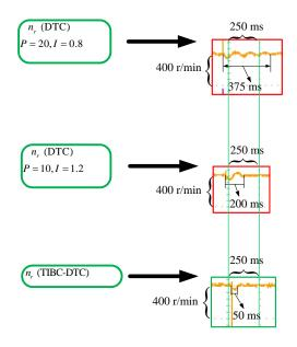
**Figure 25.** Experimental results of *n<sub>r</sub>* under DTC and TIBC-DTC.
