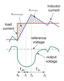
**Figure 11.** Optimal inductor current path for load current change (top: inductor current, bottom: capacitor voltage).
