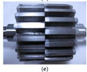
**Figure 4.** MTFTSFM: (a) The machine structure; (b) The stator structure; (c) Prototype stator; (d) The rotor structure; (e) Prototype rotor.
