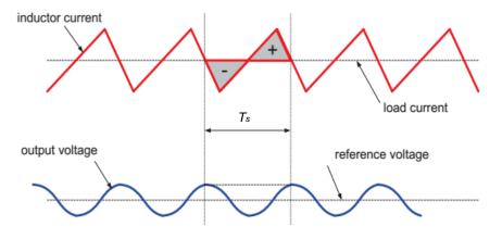
Figure 10. Waveforms of buck converter under steady-state.
