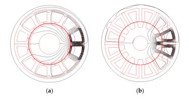
Figure 3. Armature field distribution: (a) FTRPM machine; (b) FTFSPM machine.
