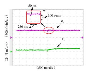
Figure 21. Dynamic performance of RDTC with TIBC (TIBC-RDTC).
