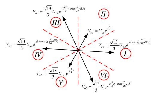
Figure 7. Reconstructed voltage vectors under phase B open-circuit fault.
