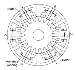
Figure 2. Fault-tolerant FSPM (MTFTFSPM) machine.
