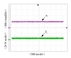
**Figure 17.**  $T_e$  and  $n_r$  of the MTFTSFPM machine under open-circuit fault using DTC.
