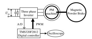
Figure 16. The diagram of test bench.
