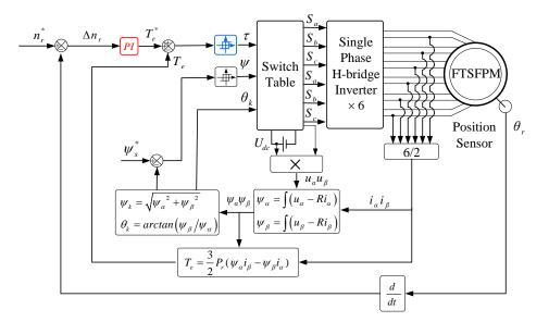
Figure 5. Diagram of the direct torque control.
