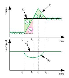
Figure 12. Optimal response to a sudden load sudden for the electromagnetic torque.
