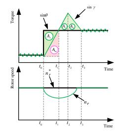
Figure 13. Optimal response to load sudden change for the torque angle.
