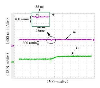
Figure 26. Experimental results of TIBC-DTC under load step change (5.5–11.5 N·m).
