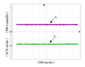
**Figure 18.**  $T_e$  and  $n_r$  of the MTFTSFPM machine under open-circuit fault using RDTC.
