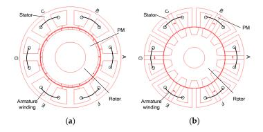
**Figure 1.** Fault tolerant PM machines. (**a**) Fault tolerant rotor-PM(FTRPM) machine; (**b**) Fault-tolerant FSPM (FTFSPM) machine.
