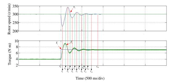
Figure 8. The dynamic process under a sudden load sudden for the direct torque control (DTC).
