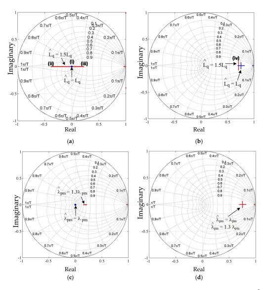
**Figure 9.** Eigenvalue (EV) migration of DB-DTFC and CVC along the U.S.06 driving cycle when  $\hat{L}_q$  and  $\hat{\lambda}_{pm}$  are detuned by 50% and 30%, respectively. (a) When  $L_q$  is detuned in DB-DTFC; (b) When  $L_q$  is detuned in CVC; (c) When  $\lambda_{pm}$  is detuned in DB-DTFC; (d) When  $\lambda_{pm}$  is detuned in CVC.
