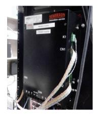
Figure 12. A Semikron power converter.
