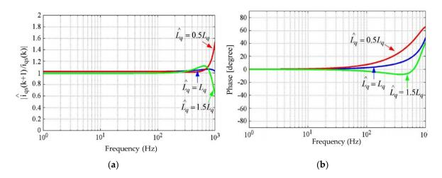
**Figure 3.** Estimation accuracy characteristic of a stator current observer with respect to q-axis inductance variation at a frequency domain [3]. (a) Magnitude of estimation accuracy; (b) Phase of estimation accuracy.
