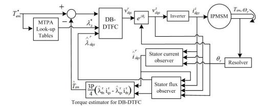
Figure 6. A block diagram of a DB-DTFC IPMSM (interior permanent magnet synchronous motor) drive.
