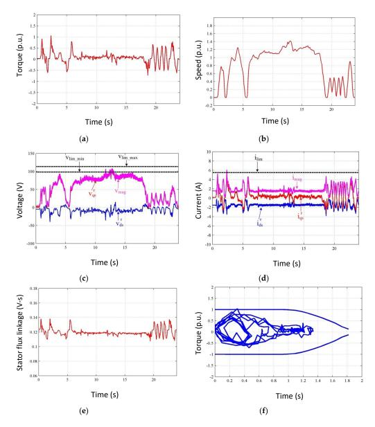
**Figure 13.** Experimental results of dynamics of the DB-DTFC IPMSM drive along the US06 SFTP driving cycle. Operating conditions:  $f_{SW} = 10$  (kHz) and  $V_{dc} = 170$  (V). (a) Torque; (b) Speed; (c) Voltage; (d) Current; (e) Stator flux linkage; (f) Torque-speed.
