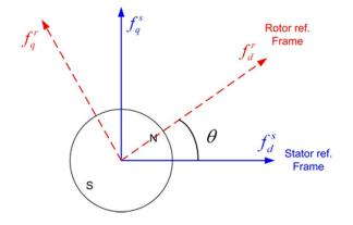
Figure 1. Stationary and rotor reference frame notation of a PMSM (permanent magnet synchronous motor).
