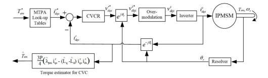
Figure 7. A block diagram of an MTPA (maximum torque per ampere) based CVC IPMSM drive.
