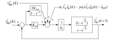
Figure 2. A block diagram of a stator current observer in a discrete time domain.
