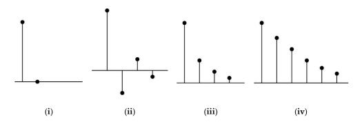
**Figure 10.** Corresponding impulse responses with respect to EV locations specified in Figure 9a,b. (i) deadbeat response; (ii) forced oscillation; (iii) underdamped response of DB-DTFC; (iv) underdamped response of CVC.
