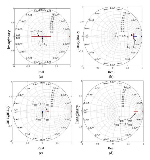
**Figure 14.** Eigenvalue (EV) migration of DB-DTFC and CVC along the US06 driving cycle when  $\hat{L}_q$  and  $\hat{\lambda}_{pm}$  are detuned by 50% and 30%, respectively. (a) When  $L_q$  is detuned in DB-DTFC; (b) When  $L_q$  is detuned in CVC; (c) When  $\lambda_{pm}$  is detuned in DB-DTFC; (d) When  $\lambda_{pm}$  is detuned in CVC.
