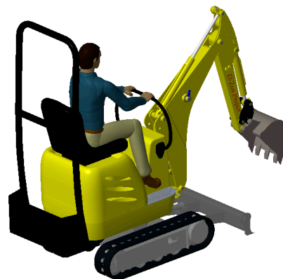
Figure 8. 3D model of the micro-excavator with a mannequin to approximate the size of the excavator.
