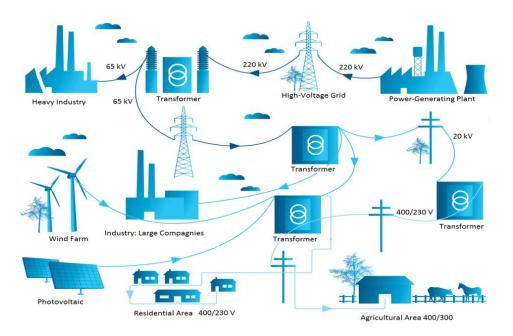
Figure 1. Schematic diagram of an electric power system.
