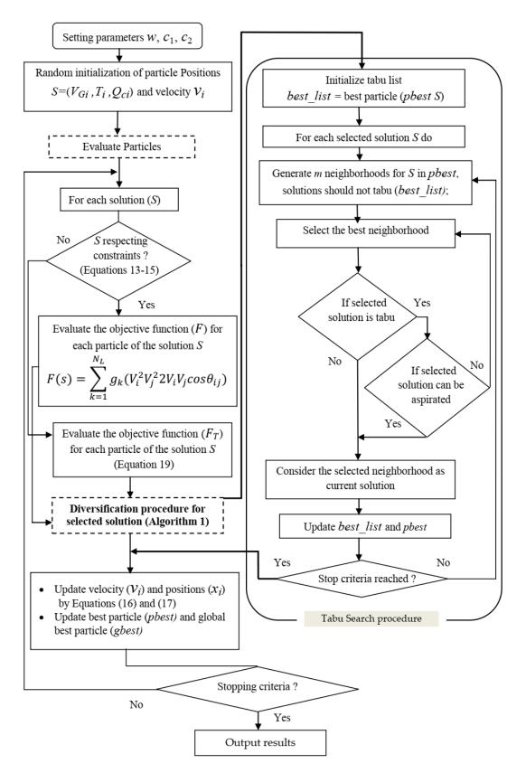
Figure 3. Detailed flowchart of the PSO-TS method.
