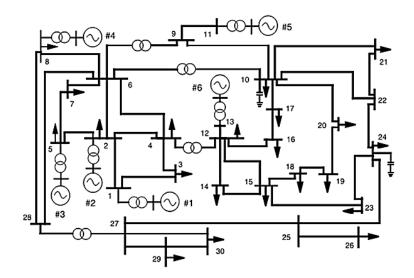
Figure 4. Single-line diagram of IEEE 30 bus test system.
