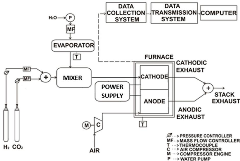
Figure 2. Lay-out of SOE stack test station.
