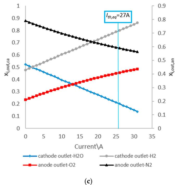
**Figure 9.** Trends of anode and cathode exhaust gas composition for the SOE stack fed by the steam mixtures 'a' (a), 'b' (b) and 'c' (c) and by air at varying the stack current.
