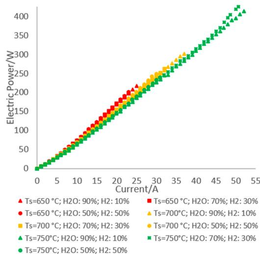
**Figure 4.** Experimental stack electric power curves in tests from 1 to 9.
