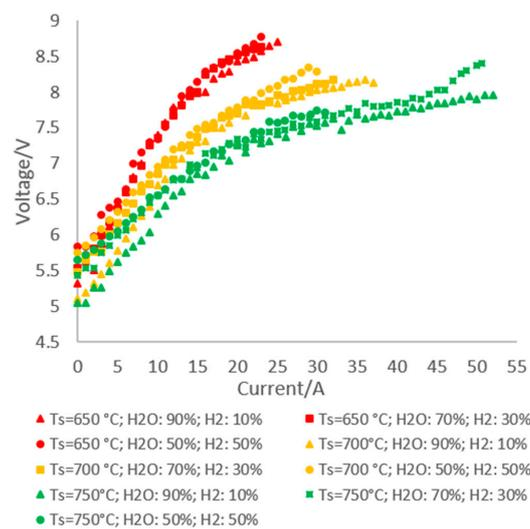
**Figure 3.** Experimental stack polarization curves in tests from 1 to 9.
