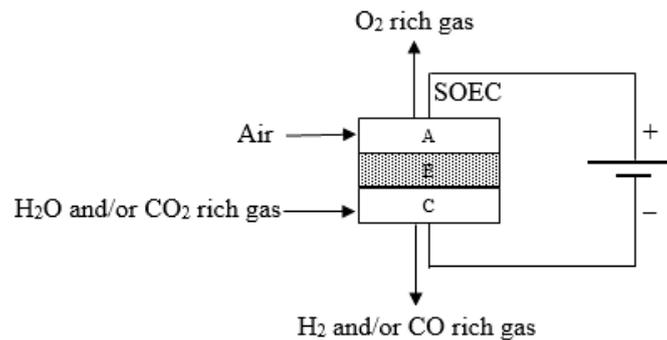
**Figure 1.** Simplified lay-out of IT-SOEC system fed by H<sub>2</sub> and/or CO<sub>2</sub> rich gas and air.
