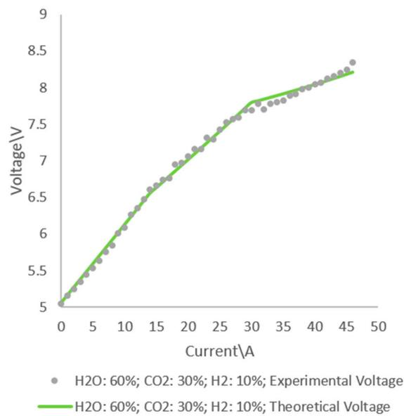
**Figure 7.** Comparison of the experimental and theoretical polarization curves of the SOE stack fed by the steam, CO<sub>2</sub> and H<sub>2</sub> gas mixture and air.
