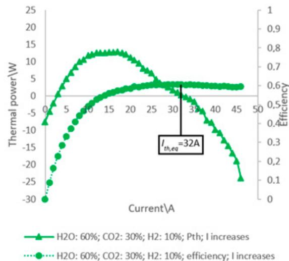
**Figure 10.** Trends of total thermal power and net production efficiency for the SOE stack fed by the steam-CO<sub>2</sub> mixture and by air at varying the stack current.
