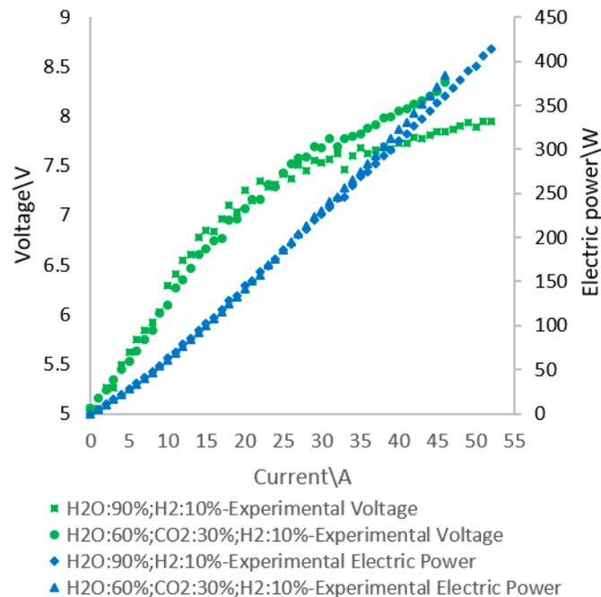
**Figure 5.** Comparison between the experimental voltage-current data and electric power-current data of the SOE stack fed by the gas mixture of steam and  $H_2$  and air and by the gas mixture of steam,  $CO_2$  and  $H_2$  and air.
