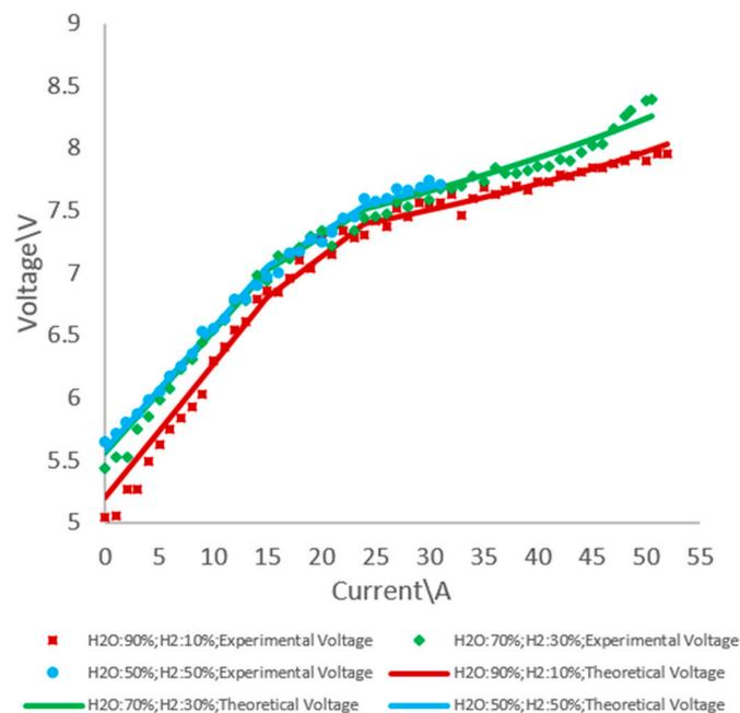
**Figure 6.** Comparison of the theoretical polarization curves and the experimental  $V_s$ - $I_s$  data of the SOE stack fed by the three different steam mixtures and air.
