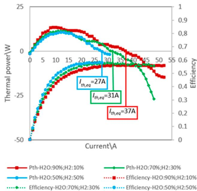
**Figure 8.** Trends of total thermal power and net production efficiency for the SOE stack fed by three steam mixtures and by air at varying the stack current.
