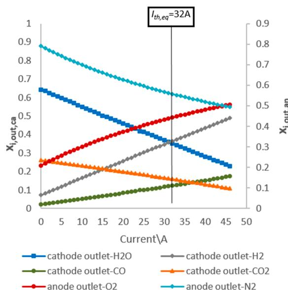
**Figure 11.** Trends of anode and cathode exhaust gas composition for the SOE stack fed the steam-CO<sub>2</sub> mixture and by air at varying the stack current.
