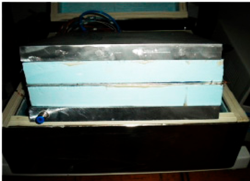
Figure 10. The assembly hot plate-specimen-cold plates.
