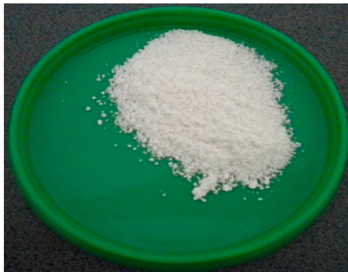
Figure 6. Polymerization result for butyl stearate microcapsules.
