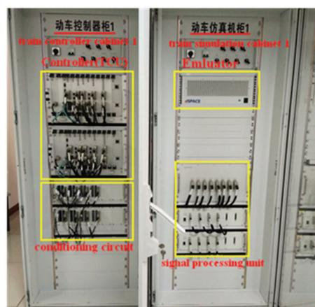
**Figure 18.** The physical diagram of the simulation cabinet.
