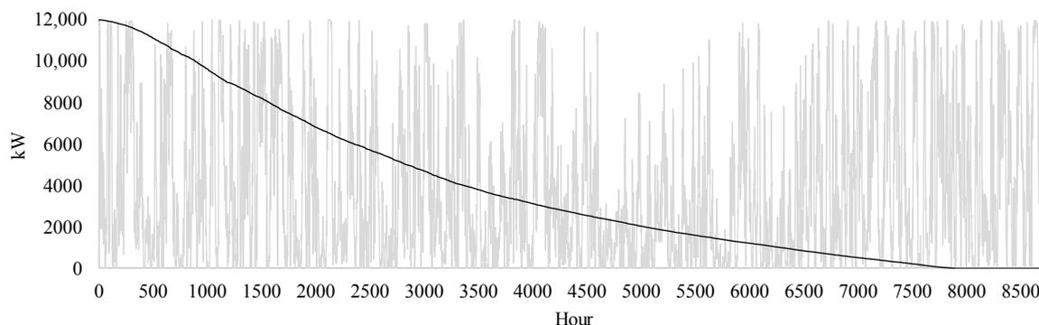
Figure 3. Summerside 2017 hourly wind generation and power duration curve.
