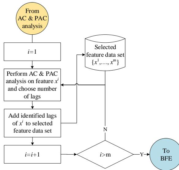
Figure 8. Autocorrelation and partial autocorrelation sub-process.
