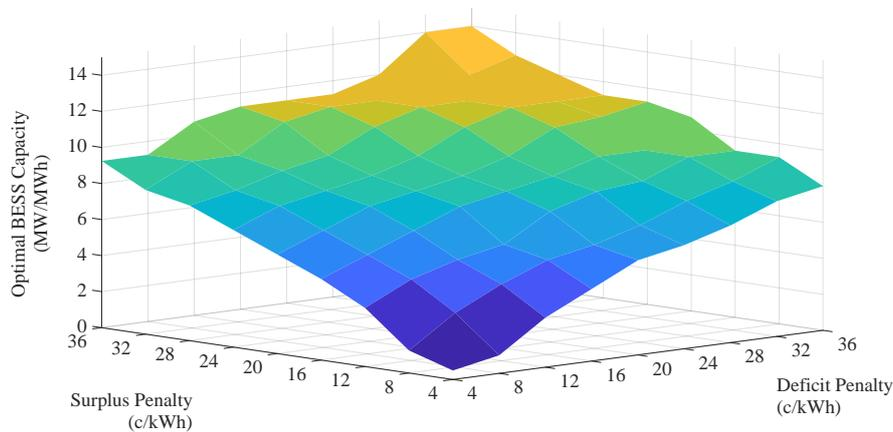
Figure 17. Optimal BESS size (MW/MWh).
