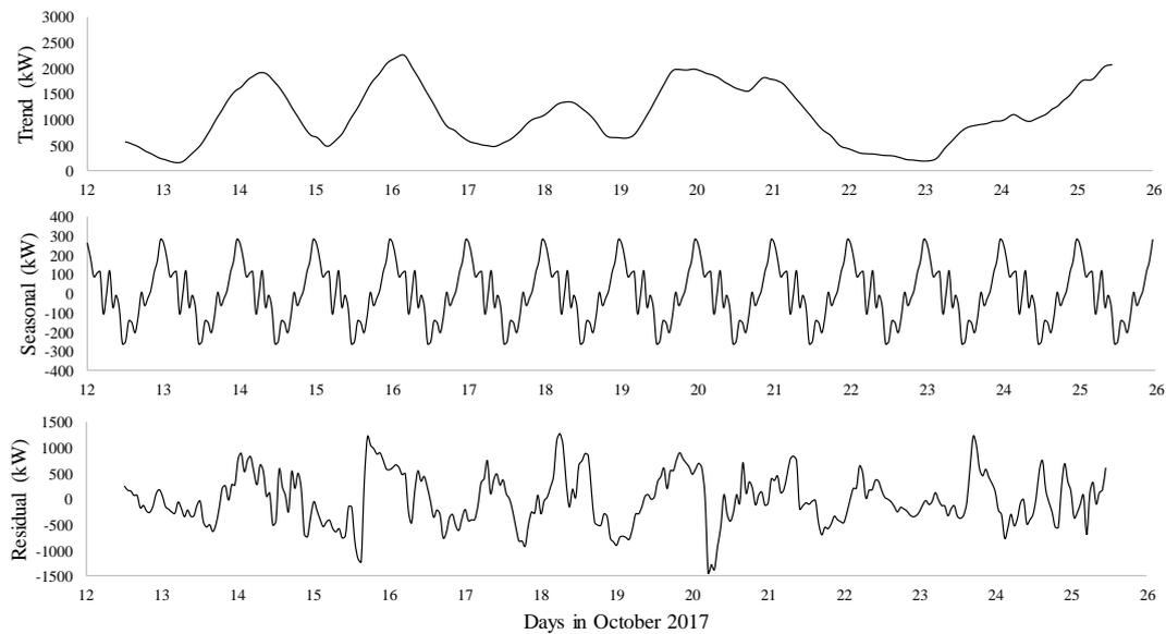
Figure 6. Wind turbine hourly output decomposition.
