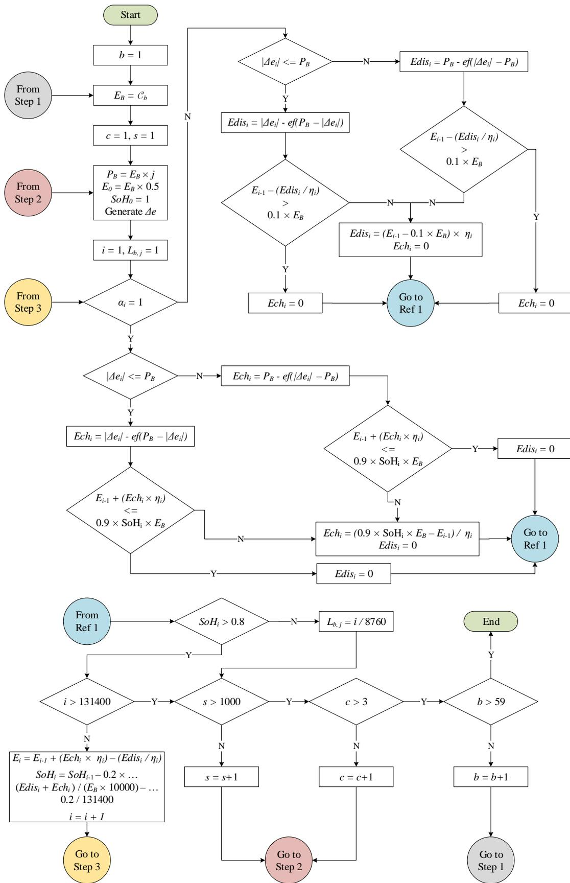
Figure 16. Flowchart of the proposed method in Section 4.2.
