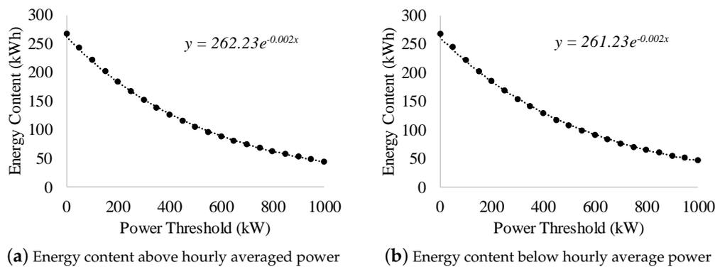
**Figure 15.** Energy above and below the averaged hourly required power vs. power thresholds.
