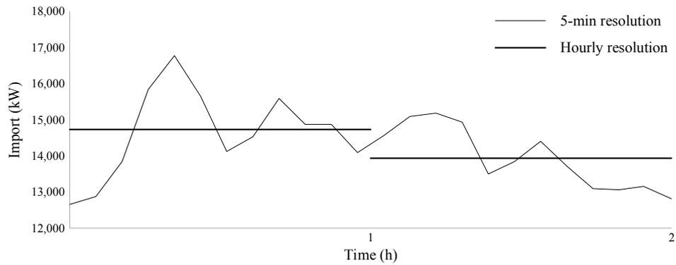
**Figure 13.** 5-min and hourly resolution of Summerside Electric actual required power import for a sample 2-h period.
