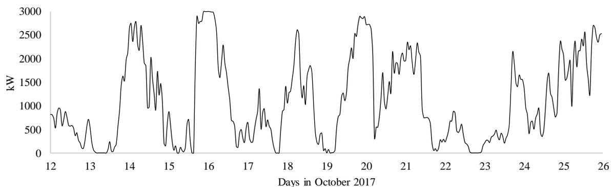
**Figure 5.** Wind turbine hourly output during a two-week period in October 2017.
