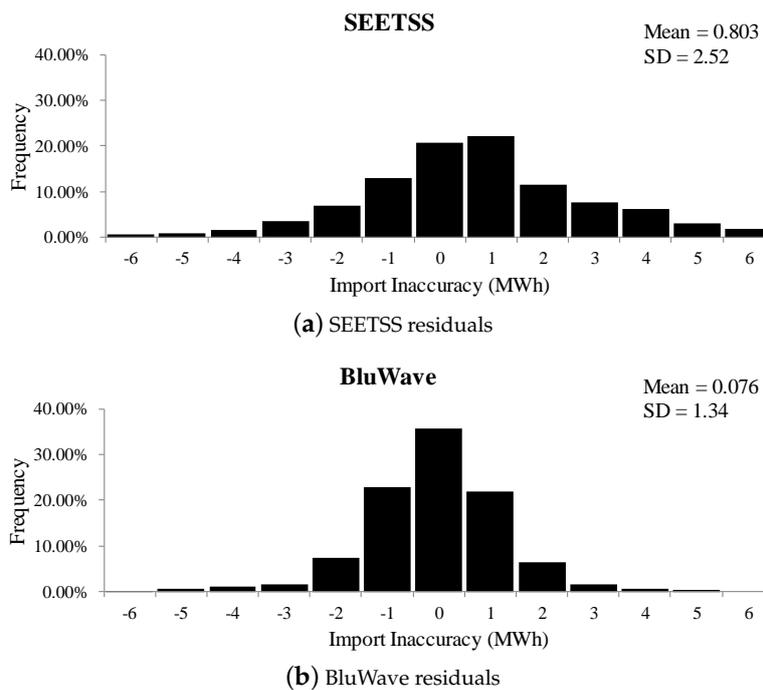
**Figure 11.** Histogram of Summerside Electric Energy Transmission Scheduling System (SEETSS) and BluWave import schedule residuals.
