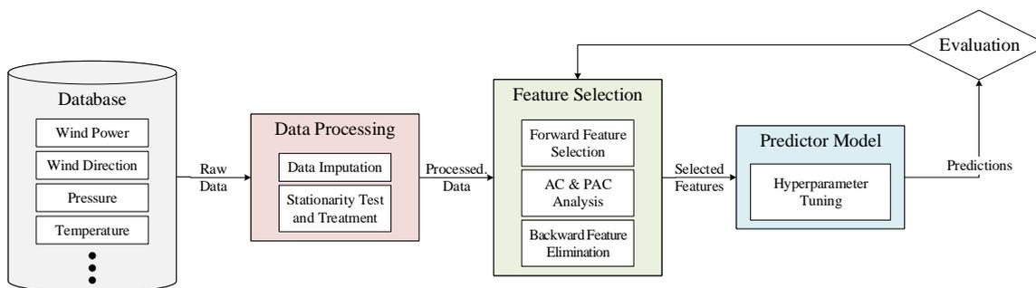
Figure 4. Schematic of wind prediction procedure.
