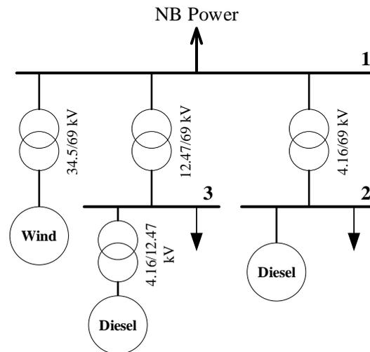
**Figure 1.** Single-line diagram of Summerside Electric grid.
