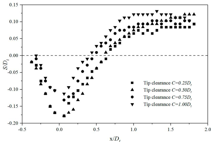
Figure 15. Scour profiles at different tip clearances.
