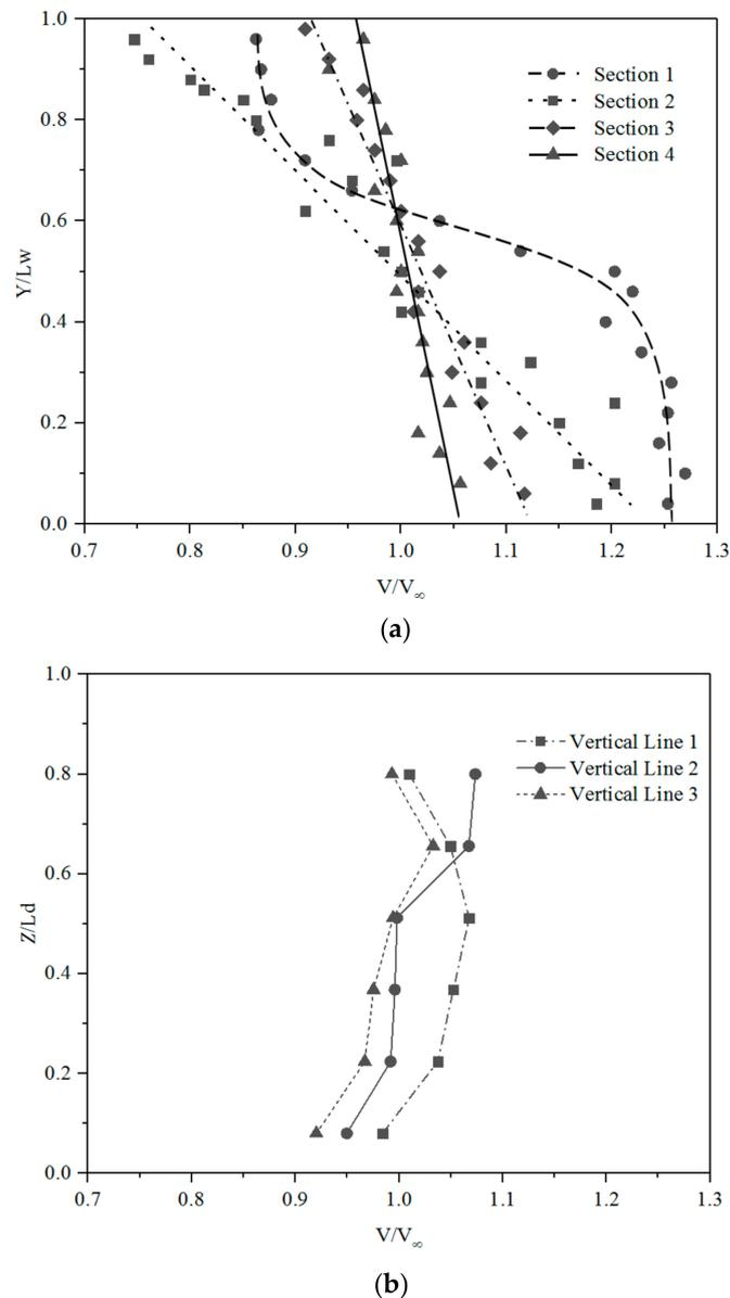
**Figure 10.** Velocity distributions at different locations: (a) Horizontal section along the channel width. (b) Vertical section along the channel depth.
