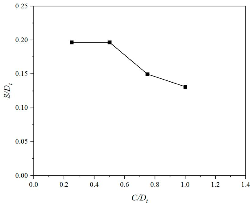
Figure 14. Seabed scour depth at different tip clearances.
