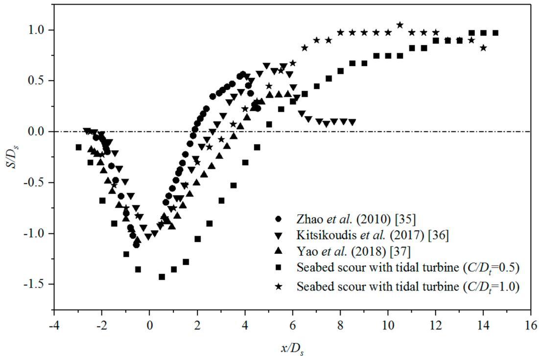
Figure 11. Tidal turbine scouring and cylinder scouring.
