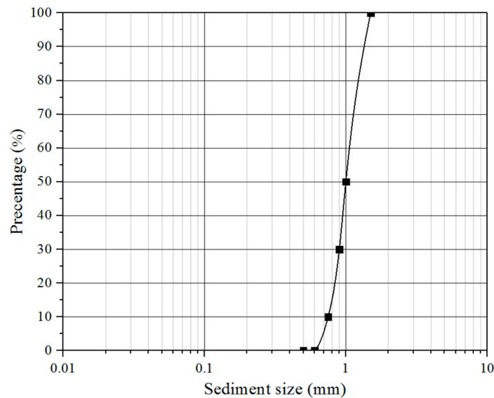
Figure 8. Particle size distribution of seabed scour sand.
