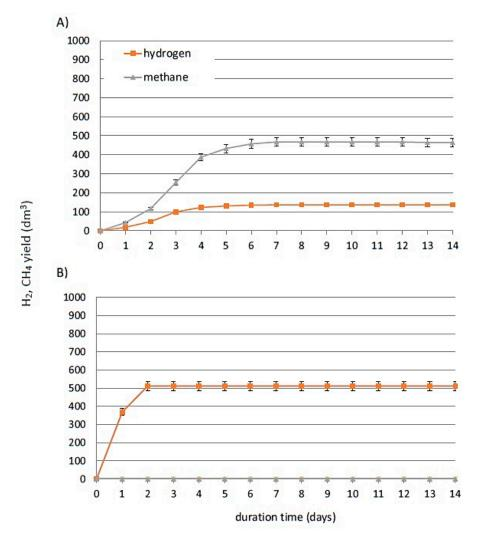
**Figure 3.** Cumulative hydrogen and methane production for TASBP-1 without pretreatment (**A**) and with pH adjustment followed by thermal pretreatment (**B**).
