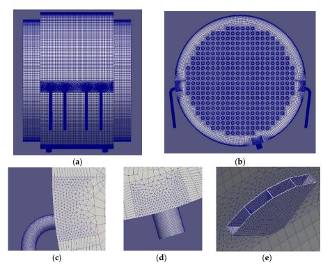
**Figure 3.** Grids of the prototype: (**a**) side longitudinal; (**b**) planform sectional; (**c**) inlet plumbing; (**d**) outlet exit; and (**d**) feeding nozzle.
