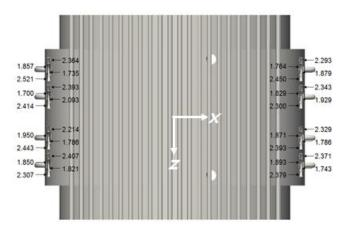
Figure 11. Mean velocities at the inlet nozzle, final time of the simulation (top view, unit: m/s).
