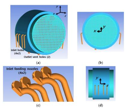
Figure 2. 3-D modeling of the prototype: (a) 3-D shape; (b) axial view; (c) feeding nozzles; (d) side view.
