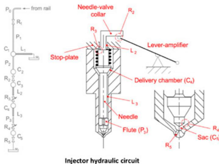
Figure 3. Schematic of the direct-acting piezoelectric injector.
