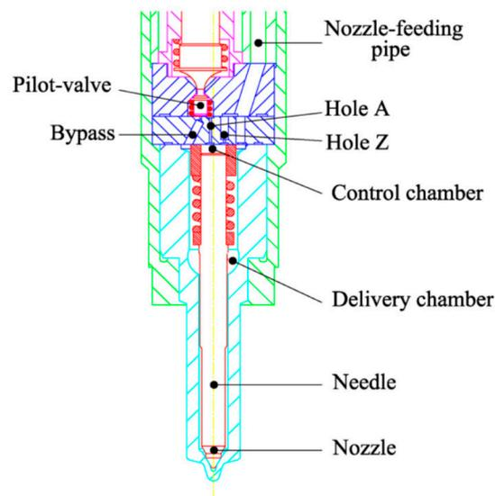
Figure 2. Schematic of the indirect-acting piezoelectric injector.
