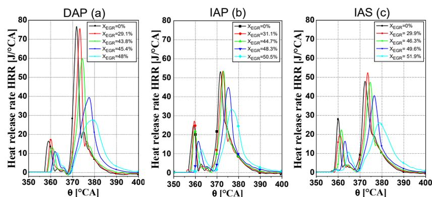
**Figure 6.** Comparison of the HRR traces featuring different EGR rates, at  $1500 \times 2$ , for the three injector typologies under investigation: (a) DAP; (b) IAP; (c) IAS.
