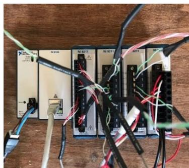
**Figure 7.** Compact Rio sensor connections.
