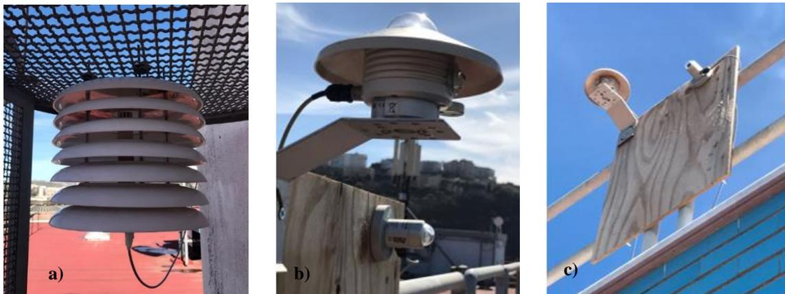
**Figure 6.** (a) Thermohygrometer in a solar radiation shield. Pyranometers: (b) side and (c) bottom views.
