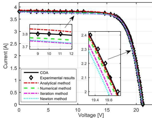
Figure 4. *I-V* characteristics of BPSolar MSX-60 module.
