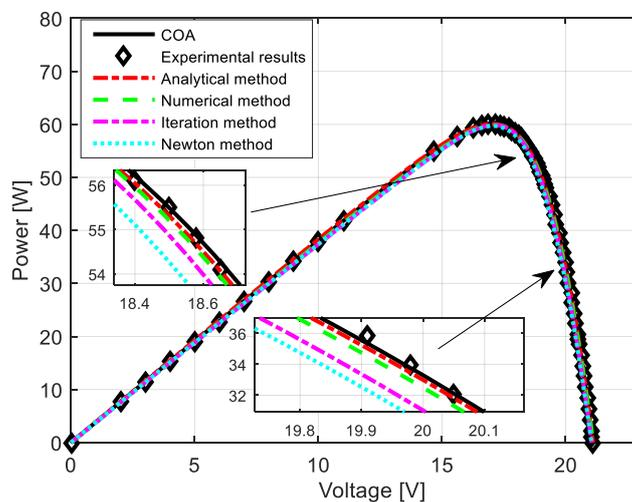
Figure 5. *P-V* characteristics of BPSolar MSX-60 module.
