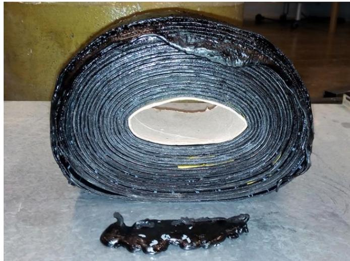
**Figure 18.** Heated asphalt roll after 8 min of heating.
