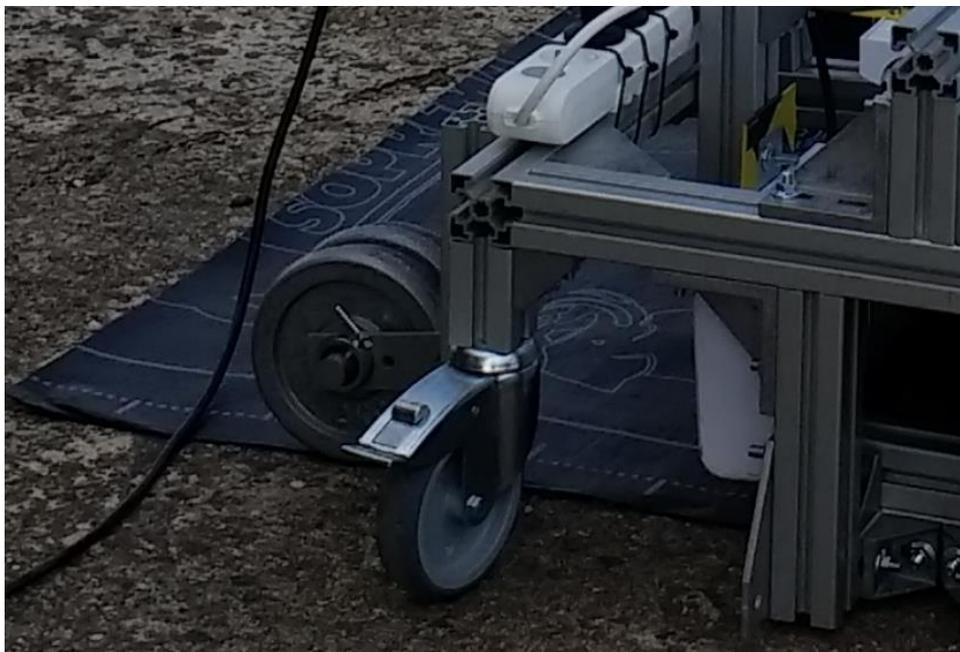
**Figure 11.** Detail of the small drum roller for the sealing of overlaps.
